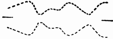
FIG. 4.—The Envelope of the Modulated Carrier.
