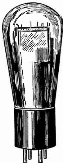
FIG. 4.—Large Type of Power Amplifier Tube.
