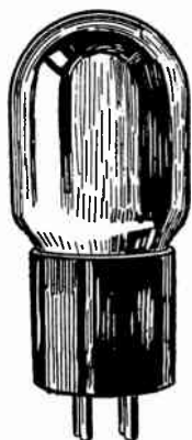
FIG. 3.—Amplifier Tube with Cylindrical Bulb.
