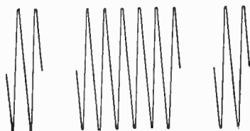
An Interrupted Continuous Wave.
