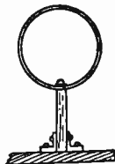
FIG. 1.—Coil Mounting in Weak Field.
