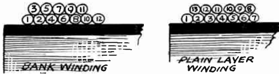
FIG. 1.—Bank Winding of Two-Layer Coil.
