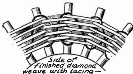
FIG. 3.—Lacing the Finished Diamond Weave Spiderweb Coil.
