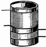
FIG. 5.—Air Core Radio Frequency Transformer.
