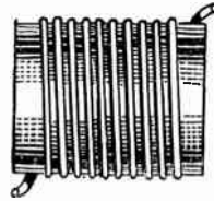
Space Winding on Single Layer Coil.
