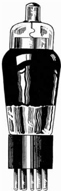
FIG. 4. — Graphite Coating on Inside of Glass Reducing Isolated Static Charges
