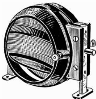
FIG. 1.—Variometer with Spherical Windings.
