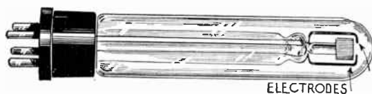
Fig. 9.—Glow Lamp for Sound Recording on Film.
