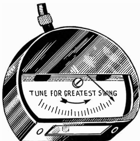
FIG. 11.—Reversed Scale Meter Tuning Indicator
