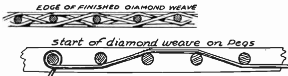
FIG. 2.—Method of Winding Diamond Weave Spiderweb Coil.
