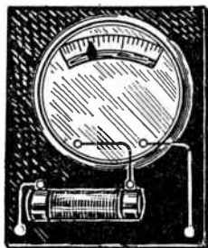
FIG. 5.—Milliammeter Used as Voltmeter.
