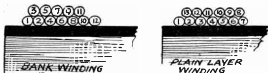
FIG. 1.—Bank Winding of Two-Layer Coil.
