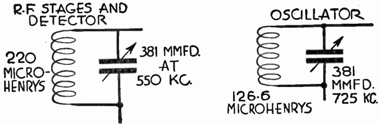
FIG. 18.—Tuning Inductances and Capacities.
