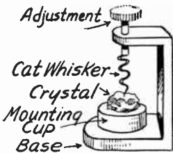
FIG. 3.—One Form of Crystal Detector.
