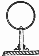
FIG. 1.—Coil Mounting in Weak Field.
