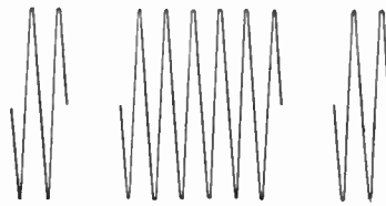
An Interrupted Continuous Wave.
