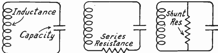
FIG. 1.—Equivalent Series and Shunt Resistances.
