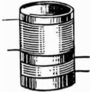
FIG. 5.—Air Core Radio Frequency Transformer.
