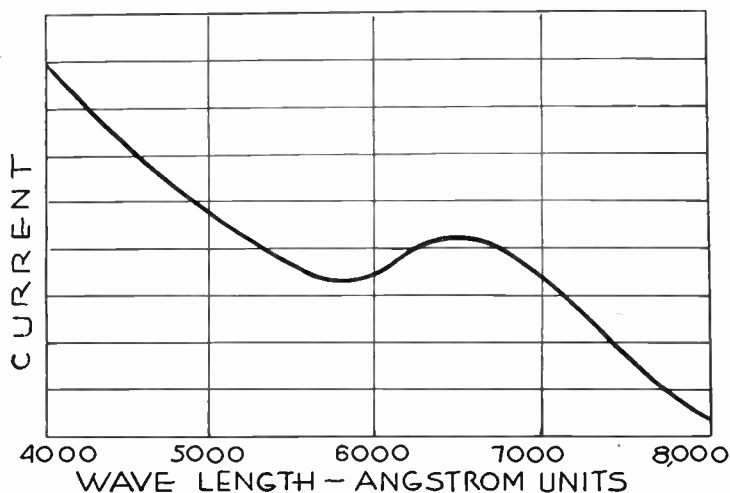
Fig. 5.—Color Sensitivity of Selenium Cell.
