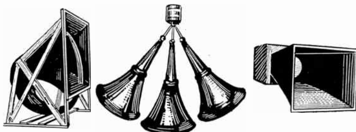
FIG. 9.—Projectors Used for Public Address Work.
