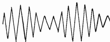
FIG. 3.—A Modulated Radio Wave.
