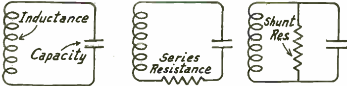
FIG. 1.—Equivalent Series and Shunt Resistances.
