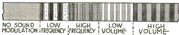
FIG. 6.—Changes in Variable Density Sound Track.
