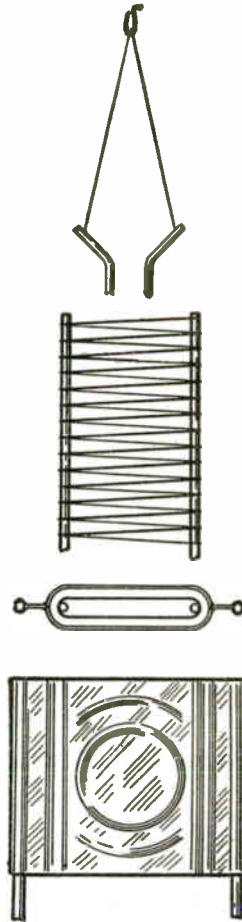
FIG. 2.—Design of Standard Type of Voltage Amplifier Tube.
