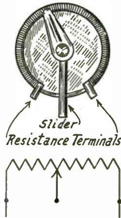
FIG. 1.—A Potentiometer and Its Symbol.
