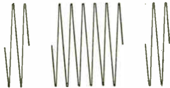
An Interrupted Continuous Wave.
