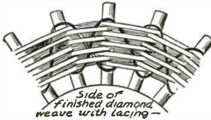
FIG. 3.—Lacing the Finished Diamond Weave Spiderweb Coil.
