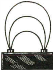
FIG. 1.—Circuits with Resistances in Parallel on Battery.
