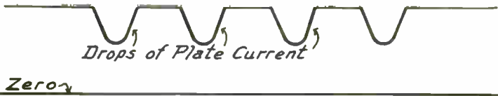
FIG. 13.—Drops of Plate Current Due to Decreases of Grid Voltage in Tube.
