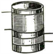
FIG. 5.—Air Core Radio Frequency Transformer.
