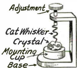
FIG. 3.—One Form of Crystal Detector.
