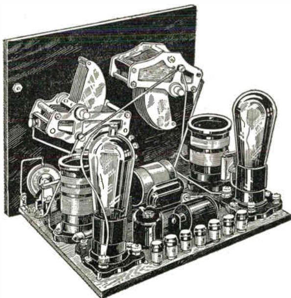
FIG. 8.—Arrangement of Parts in Simple Converter.
