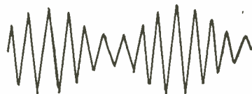
FIG. 3.—A Modulated Radio Wave.
