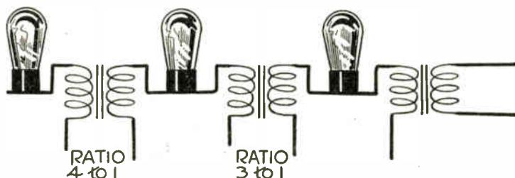
FIG. 2.—Power Tube Overloading.
