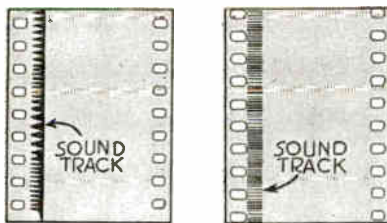
FIG. 2.—Sound Tracks with Variable Area (left) and Variable Density (right).
