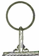
FIG. 1.—Coil Mounting in Weak Field.
