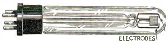
FIG. 9.—Glow Lamp for Sound Recording on Film.
