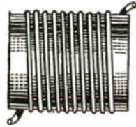
Space Winding on Single Layer Coil.
