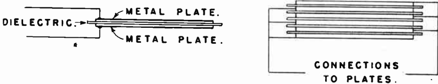
Fig. 61. A capacitor consists of insulating material, called the dielectric, between conductive plates of metal.
