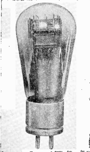
Fig. 8. A pliotron which will operate as an oscillator or as an amplifier.
