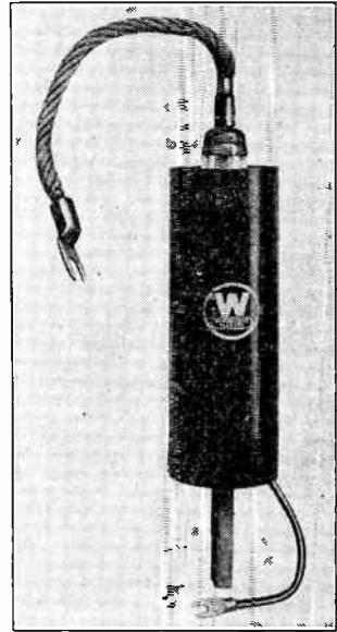
Fig. 316. A welding ignitron WL-652 rated for a maximum demand of 600 kilovolt-amperes.
