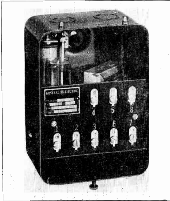
Fig. 325. Accessible terminal connections on a relay. The electromagnetic relay is back of the tube. The heater transformer is at one side.
