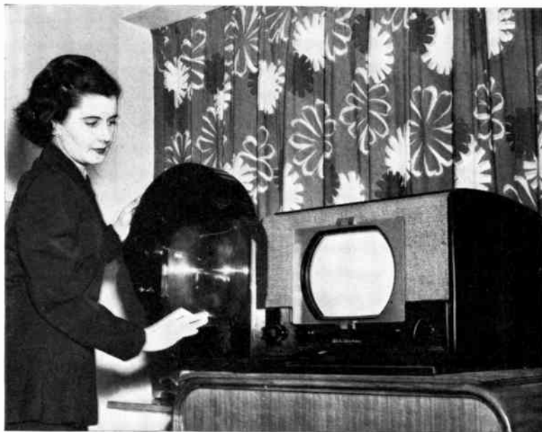
Fig. 5.—Table model standard black-and-white television set with a scanning adapter which will enable it to get CBS color television signals in black-and-white, in addition to getting standard black-and-white signals in black-and-white.
