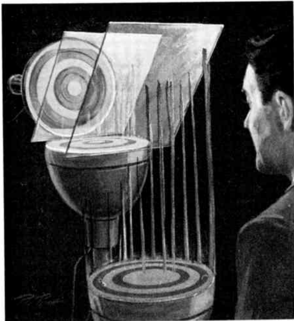
Fig. 8.—RCA direct view color reproduction system using three kinescopes and two dichroic mirrors.
