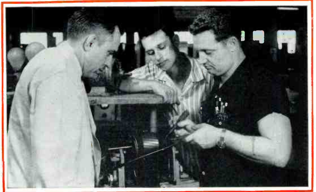
The picture above shows an Instructor giving instruction on a special growler designed to test armatures with specialized windings. This growler was invented by a Coyne Graduate and is produced by a nationally known Manufacturer.
