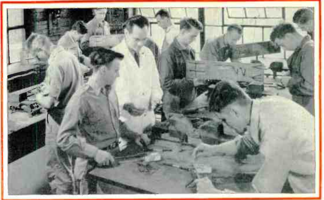
This picture shows a group of students getting started with their jobs that will give them practice in wire splicing and soldering with gas heated soldering coppers. This is the kind of training that fits a fellow to do practical work out on the job.
