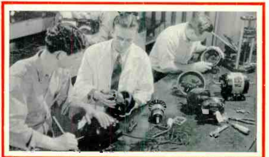
Here you see students reaming bearings and checking motors of the types commonly used on many popular Household Appliances.
