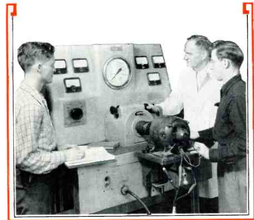
These Coyne students are testing the efficiency of a motor with a modern Dynamometer, a type used extensively in industry for testing A.C. and D.C. motors.
