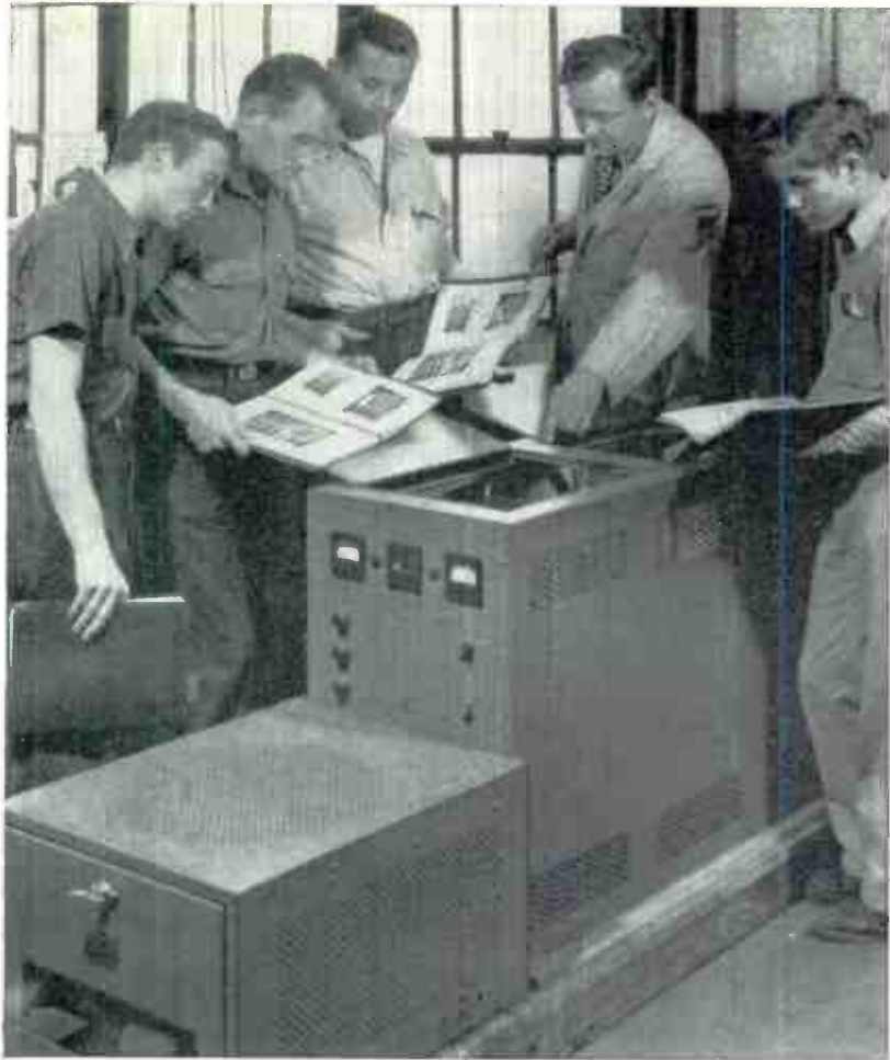
This picture shows students getting instruction on the operation of a Dielectric Heating unit used in plastic moulding and sealing of Vinylite material for raincoats, aprons, tablecloths, etc.
