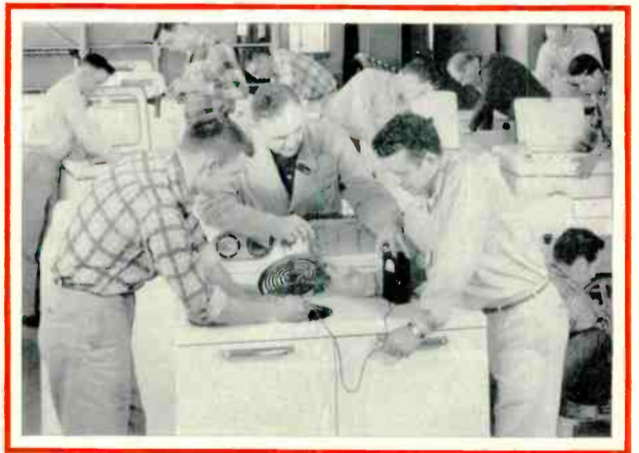
Here is an Electric Range with automatic temperature and timer equipment. Students are getting instruction on making efficiency tests and where to look for troubles that might develop in such equipment.
