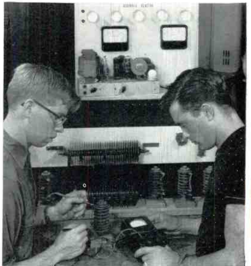
The Students below are testing rectifiers of the type used in Resistance Welding equipment, Magnetic Chucks and Electronic Instruments. Solid-State Rectifiers are replacing vacuum and gaseous type Rectifiers in many Industrial Electronic Circuits.
