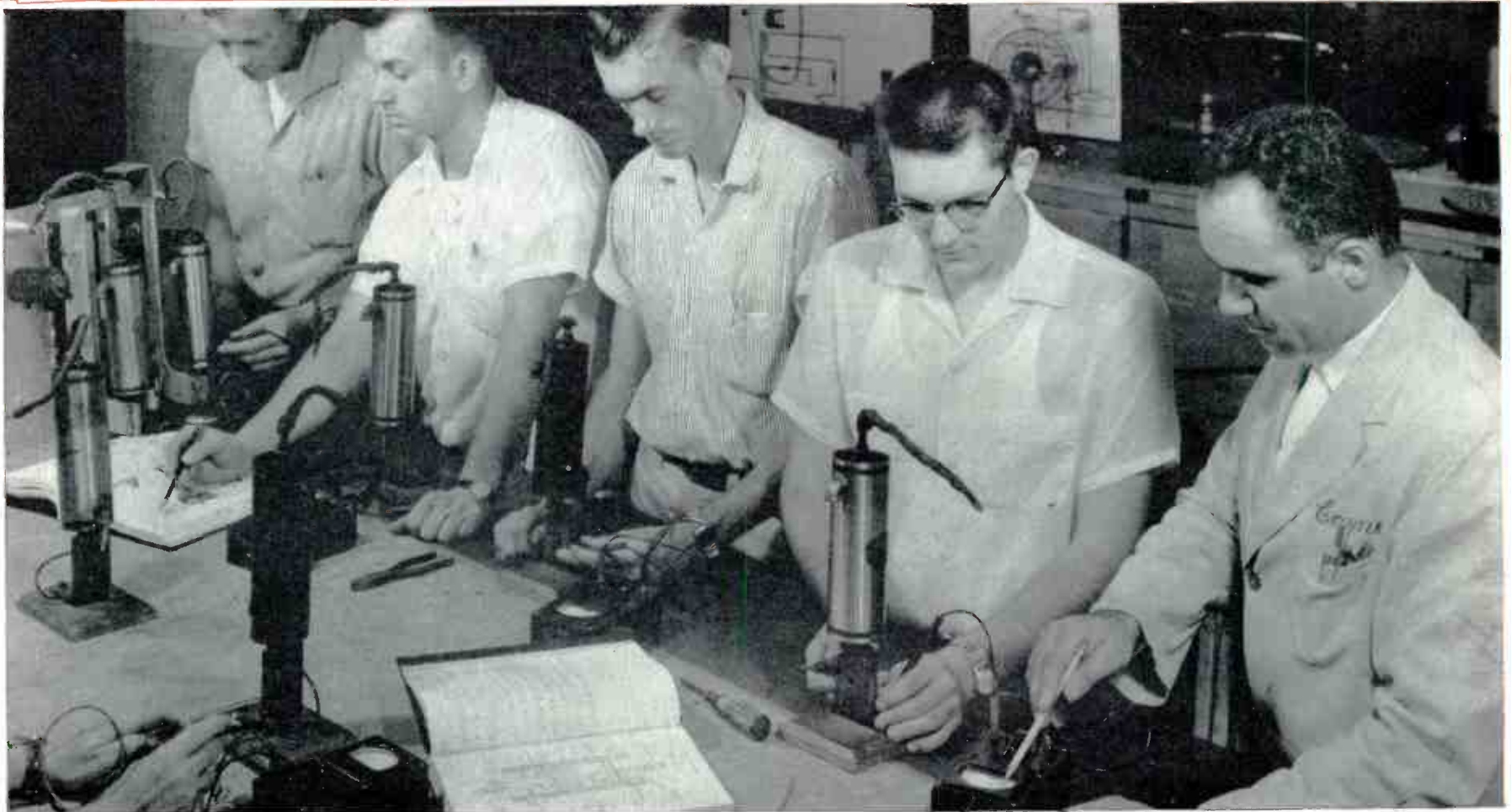
The Ignitron Tube has proved invaluable for use in Electronic Switches, welding controls, and many other applications. The photo below shows students getting practical experience and instruction in the operation of this Electronic Tube.
