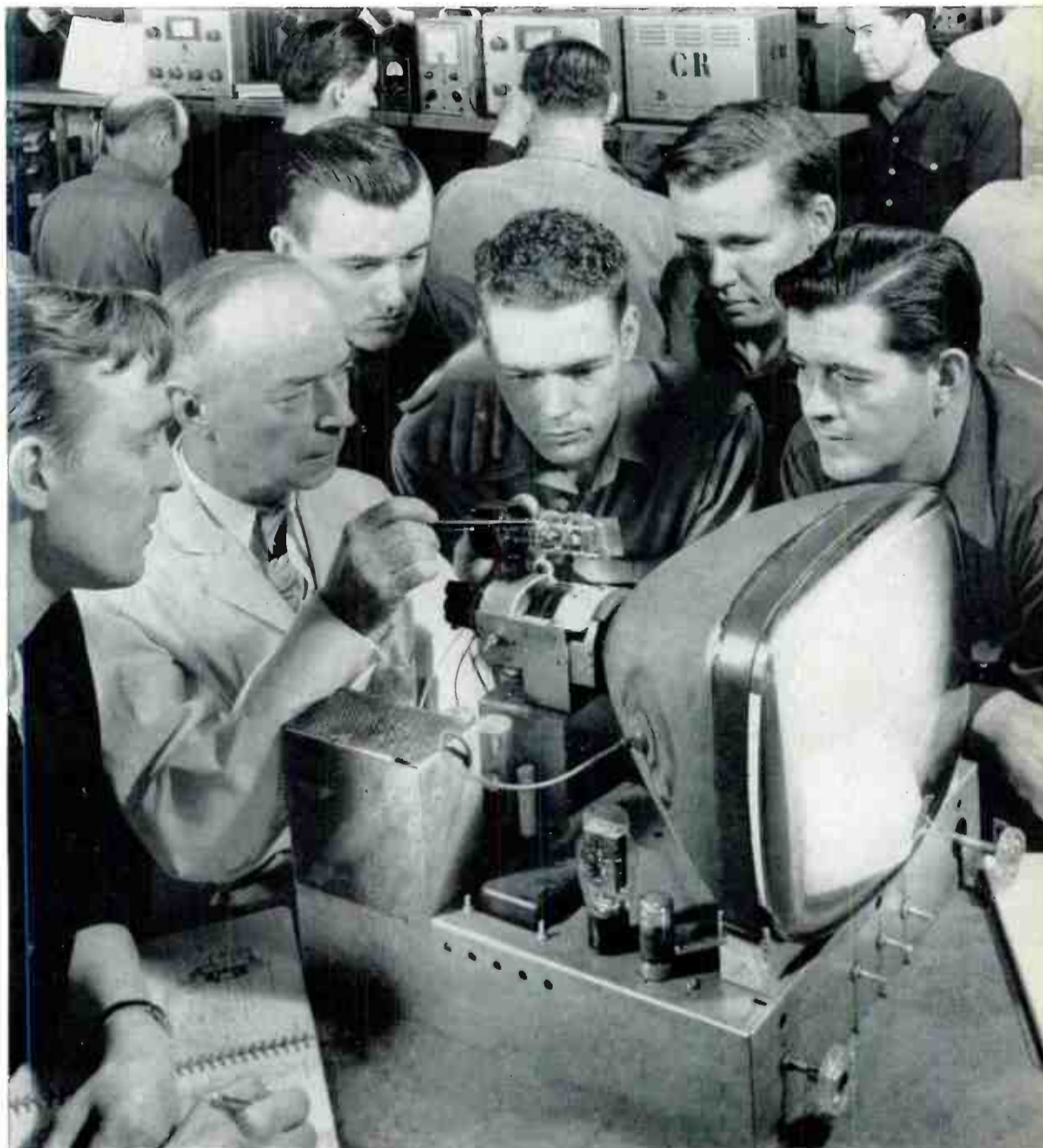
This photo shows an instructor giving a demonstration and explanation on how basic principles are utilized in the electron gun of a Television Picture Tube. The electron gun is the heart of a Cathode Ray Tube used in Television.
