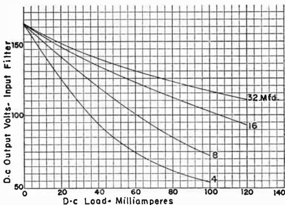
Fig. 11-4. Effect of various capacitances in first filter capacitor.
