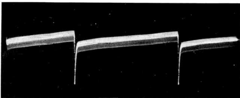
Fig. 10-20. Voltage waveform at vertical yoke coils connected to a plate coupled multivibrator.
