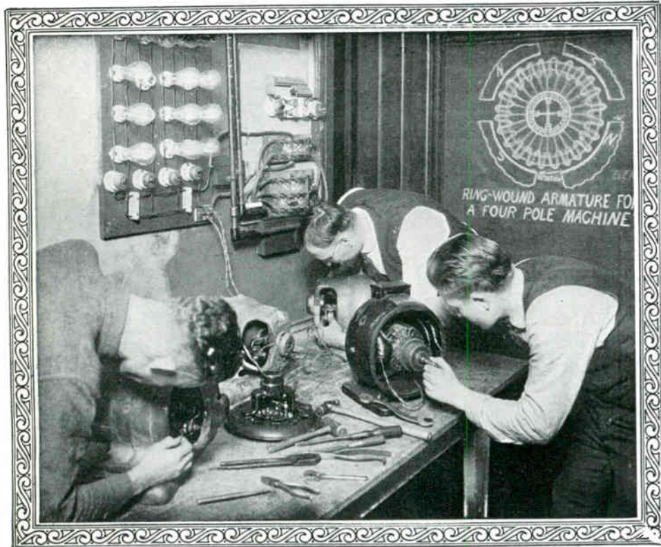
Assembling and Testing Re-wound Armatures
