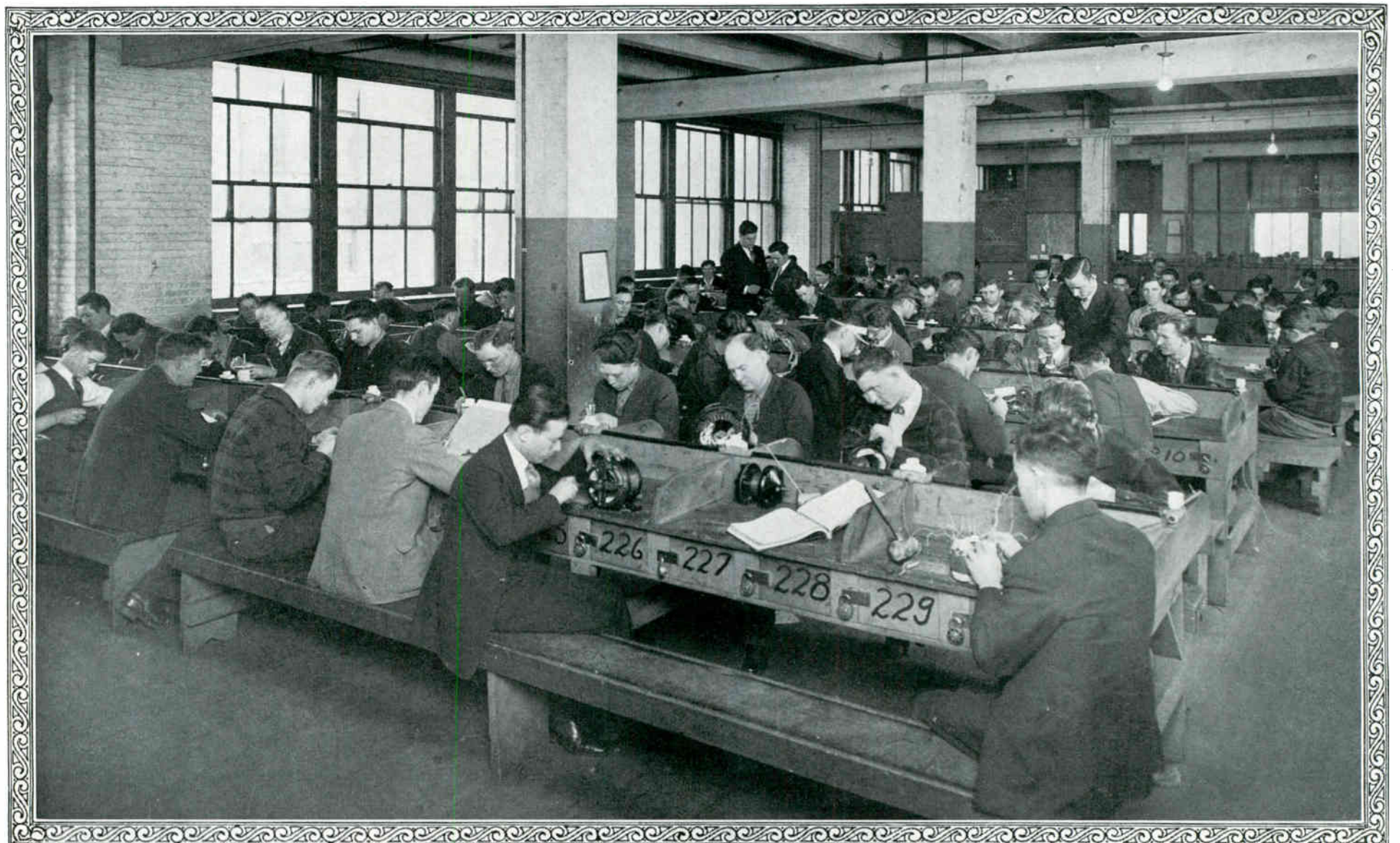
A Part of the Armature Department Showing Students Doing Actual Wire Winding on Armatures and Stators
