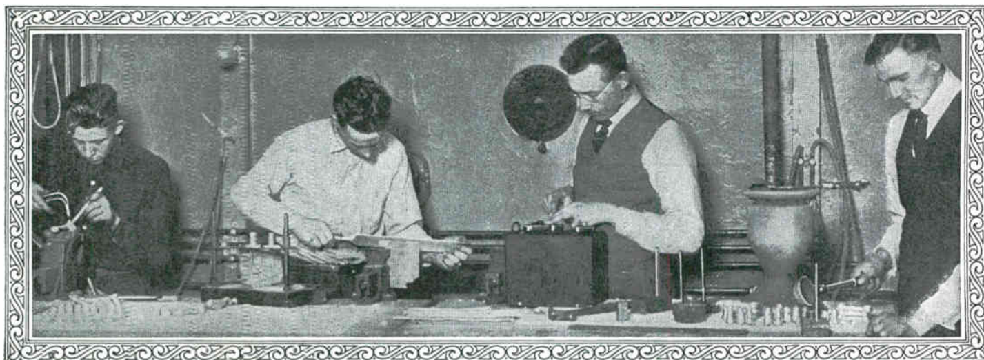
Students Acquiring Speed in Battery Repairs. Tearing Down and Rebuilding a Modern 3-Cell, 6-80 Battery
