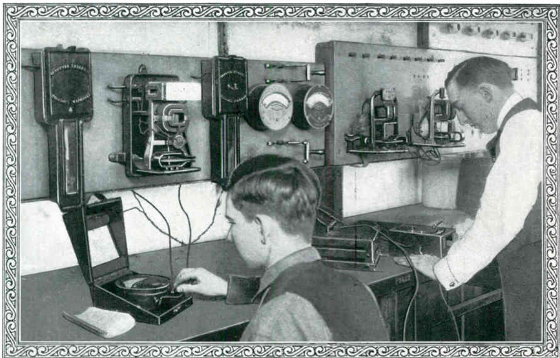
Learning by Doing—Testing Watt Meters
