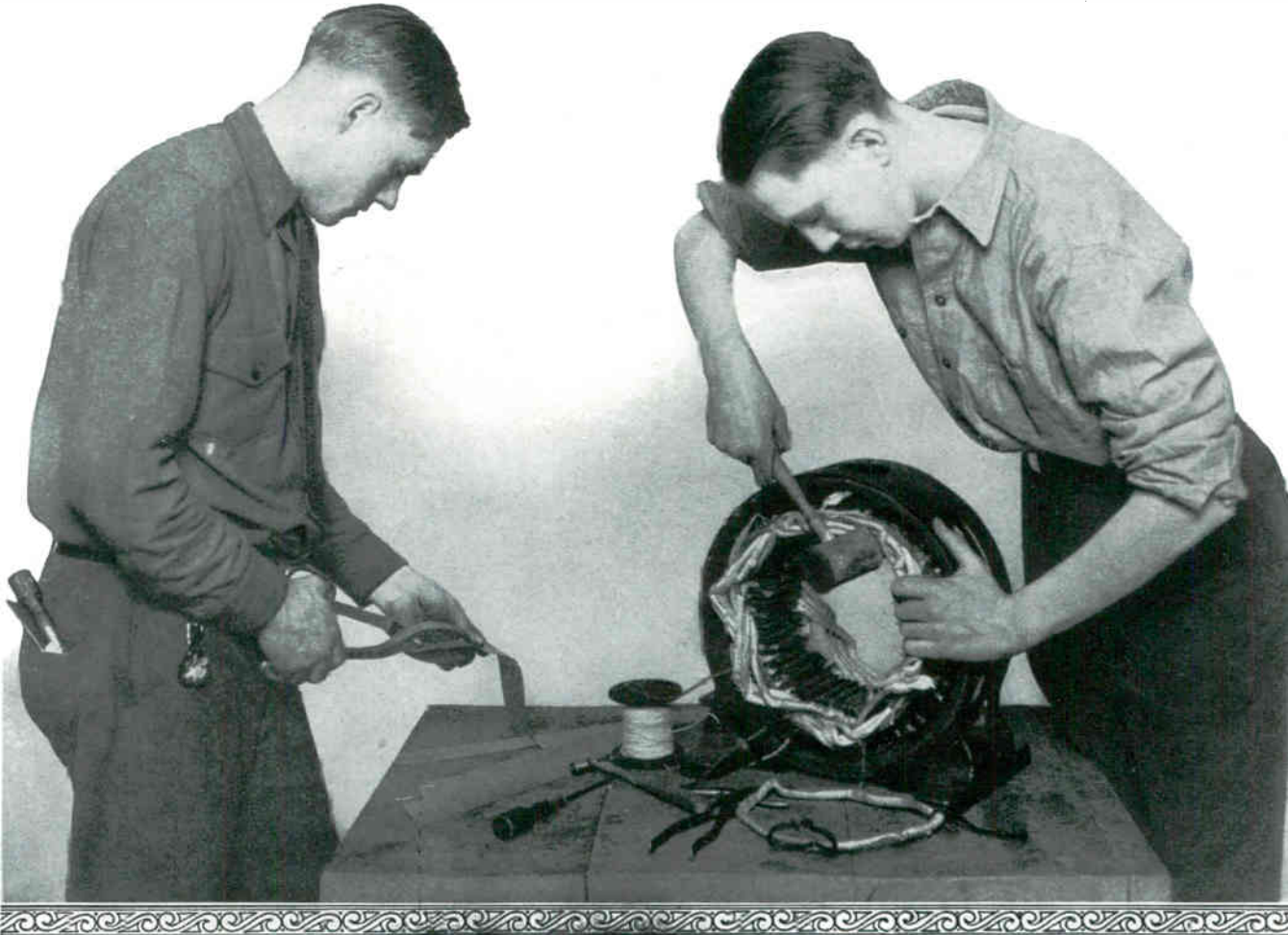
Overhauling and Testing a Motor Before Rewinding
