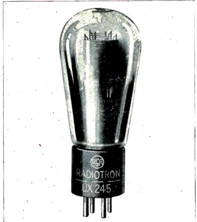
Fig. 75. Photo of power amplifier tube such as used for obtaining great amplification and handling larger amounts of plate current for producing stronger signals from radio receivers. (Photo courtesy of R. C. A. Radiotron Co., Inc.)
