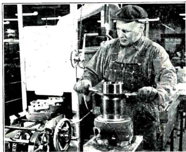
Fig. 153. Assembly operation on cylinder head and barrel of radial Diesel engine.
