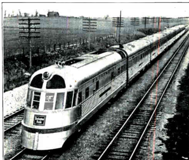
Fig. 89. Modern high speed Diesel Electric Train. The operation of trains of this type is made possible through the economy and efficiency of the Diesel engine, plus the flexibility and ease of control of the electric generator and electric driving motors. (Courtesy Burlington Railway Co.)
