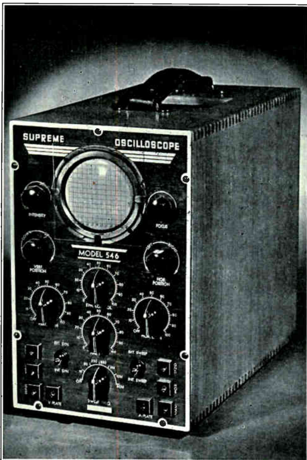
Fig. 245. Photograph of a modern cathode ray oscilloscope of a type now becoming very popular as a radio service instrument. Note the end of the cathode ray tube near the top center of the panel. Also note the various control knobs and switches used for adjusting and operating this instrument. Courtesy Supreme Instrument Company.
