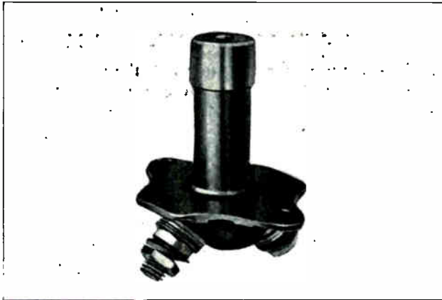
Fig. 79. Starter switch for mounting on the floorboard and connecting in series with the lead from the battery to the starting motor.
