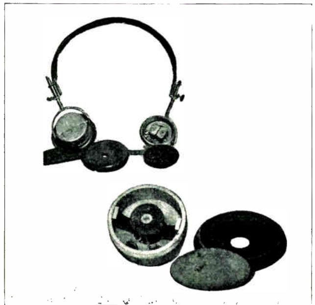
Fig. 126. The top photo shows a pair of phones with the cover and diaphragm removed from one to show the magnets, and below is shown an open view of a single large phone unit for use on a speaker horn.
