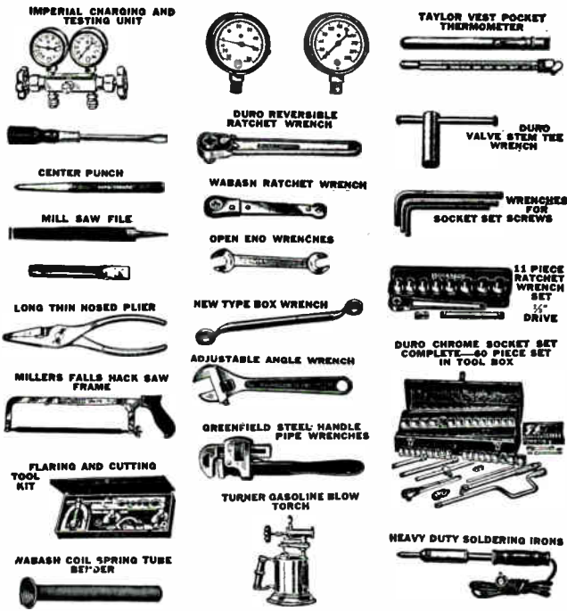
Fig. 120. Above are shown some of the most commonly used refrigeration service tools.
