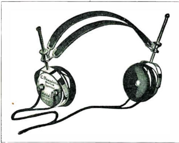
Fig. 125. This photo shows a pair of earphones or headphones as they are often called. Phones of this type are very useful for receiving weak signals that are not strong enough to operate a speaker, and also for testing radio devices and circuits.
