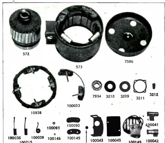
Fig. 112. This view shows the important parts of a disassembled refrigerator motor of the repulsion-induction type. Courtesy Kelvinator Corp.
