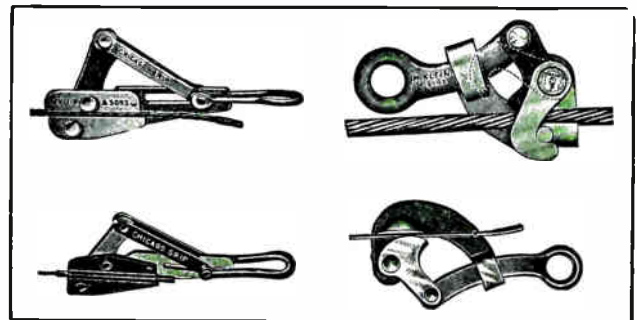
Fig. 364. Several different types of "come-alongs" or pulling grips used for drawing up conductors or transmission lines.
