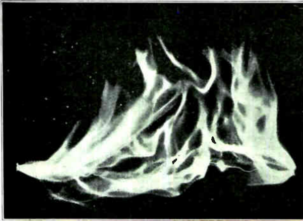
Fig. 2. The above view shows a high voltage arc created by passing current at a potential of several hundred thousand volts through air.
