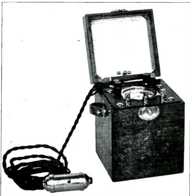
Fig. 66. Watthour test meter or rotating standard, used for calibrating watthour meters.
