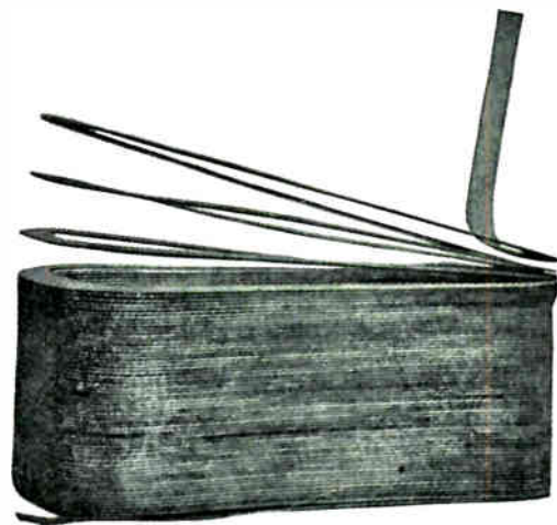
Fig. 89. Field coil which is wound with thin copper strip, making a coil which is very compact and easily cooled.
