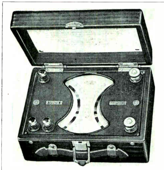
Fig. 51. This portable meter has two elements and two scales, and can be used to measure either volts or amperes. The voltmeter element has an extra terminal to provide increased voltage range of this instrument. (Photo courtesy Jewell Instrument Company.)
