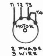
2 PHASE 3 WIRE L3 IS COMMON LINE
