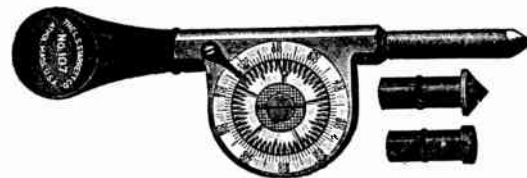
Fig. 472. Revolution counters or speed indicators of the above type are very convenient for checking the speeds of motors and generators.
