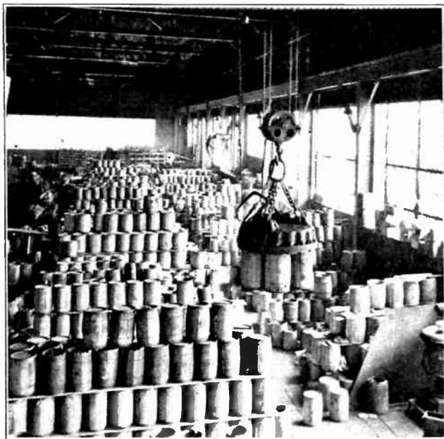
Fig. 8. Direct current is used to operate powerful electro-magnets of the above type for handling metal materials in industrial plants, warehouses, foundries, and iron yards. Note the manner in which these kegs of bolts are lifted by the magnet, even though the wooden heads of the kegs are between the magnet and the metal to be lifted. In plants where the principal supply of electricity is alternating current small motor generators are often used to supply the direct current for magnets of this type.
