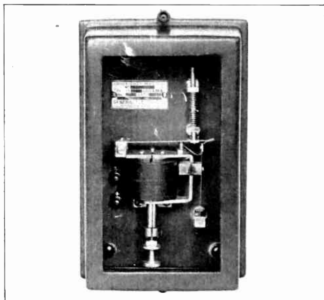
Fig. 437. Photo of a high-voltage cutout relay clearly showing the coil and contacts. Courtesy of G. E. Company.
