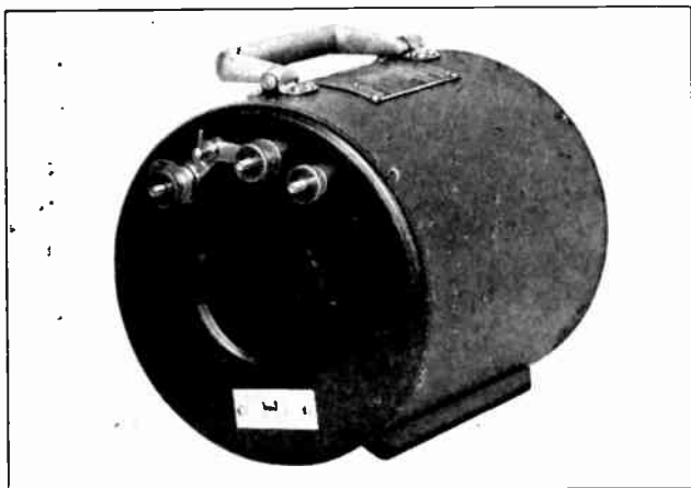
Fig. 146. Portable current transformers of this type are very convenient when making tests on lines or electric machines with portable ammeters and wattmeters. (Photo Courtesy General Electric Co.)
