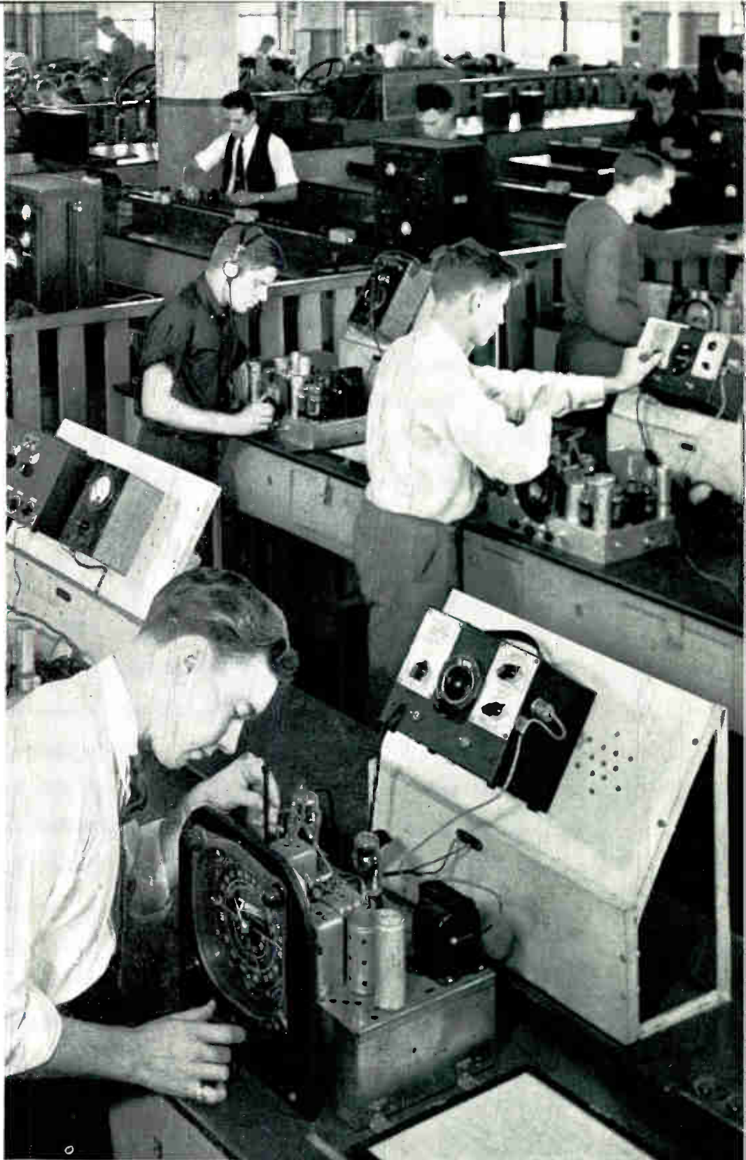
Students testing and aligning modern all-wave receivers with oscillators and cathode ray oscilloscope. Training on such up-to-date equipment helps fit you for the better paying jobs in radio.
