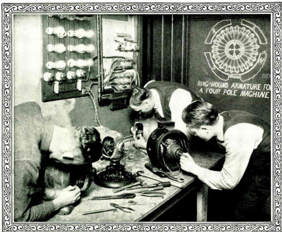
Assembling and Testing Re-wound Armatures
