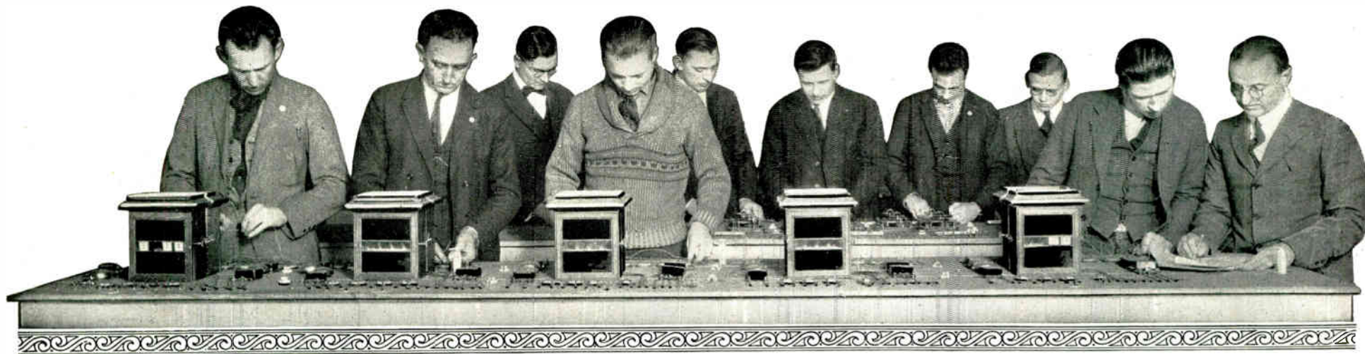
Students Wiring Annunciators and Testing Out Various Kinds of Circuits—This Is Fascinating Work
