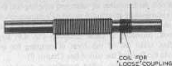
Fig. 4.9 'Loose' inductive coupling with separate coupling coil.
