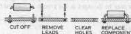
Fig. 12.12 Remaining leads can then be removed, ready to fit new component.
