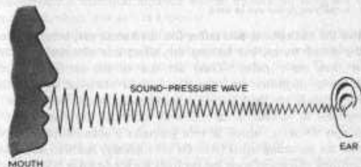
Fig. 1.1 Speech is transmitted directly through the air by sound-pressure waves.
