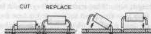
Fig. 12.11 The safest way to remove a faulty component is usually to cut it off.
