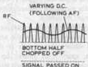
Fig. 1.12 The form of the signal passed by a diode detector—a mixture of 'chopped' RF and a d.c. component varying in AF.
