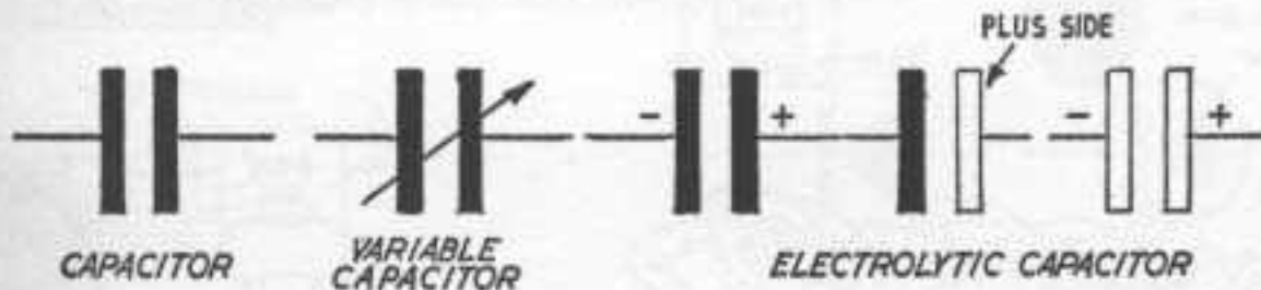
Fig. 11. The symbols which may be used to designate capacitors on a circuit drawing. In practice, all capacitors from 0.1 microfarads up are electrolytic type
