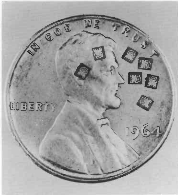
Courtesy Sylvania Electric Products, Inc. Fig. 1-7. Seven complete IC chips on a penny.
