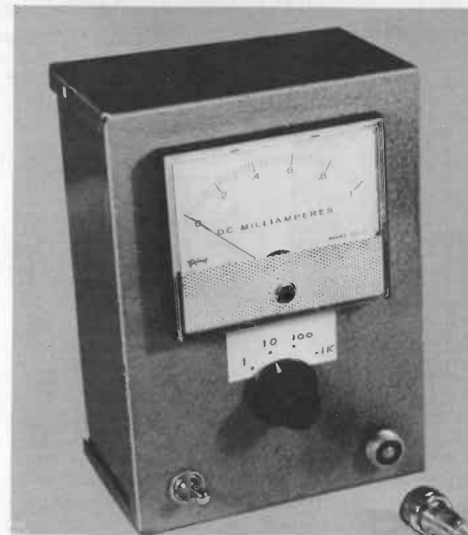
Fig. 8-1. Overall view of the electronic DC voltmeter.
