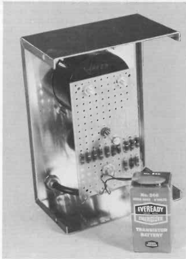
Fig. 8-2. Inside view of the electronic voltmeter.
