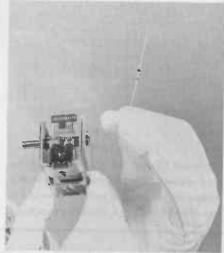
THIS TINY VARIABLE CAPACITY DIODE WILL REPLACE THE CAPACITORS
