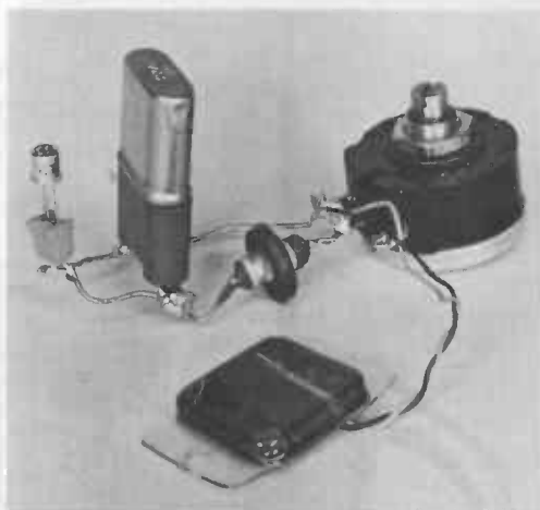
A solar operated 80 meter c.w. transmitter. The solar cell, in the foreground, is an International Rectifier SD-1020-A.
