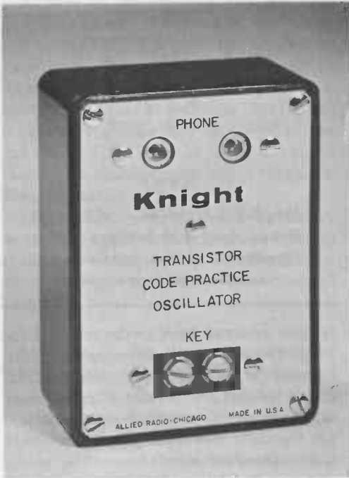
THE KNIGHT CODE PRACTICE OSCILLATOR This oscillator is a simple tickler coil audio oscillator similar to Fig. 3.8-A. (Photo by Allied Radio)
