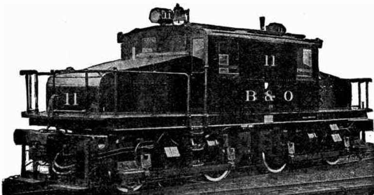
FIG. 3,646.—General Electric 100 ton locomotive for moderate speed heavy passenger and freight service. There are four 300 horse power motors of the box frame, commutating pole forced ventilated type. Each of these motors at its one hour rating will develop a torque of 4,000 lb. at a one foot radius. The gearing between the motor and driving axle has a 4.37 reduction and the driving wheels are 48 in. in diameter. With this reduction each motor will develop a tractive effort of 8,750 lb. at the rail head, which gives a total tractive effort for the four motors of 35,000 lb. This tractive effort will be developed at a speed of 12 miles per hour. The four motors have an overload capacity sufficient to slip the driving wheels and can develop under maximum conditions a momentary tractive effort of 50,000 lb. to 60,000 lb. The maximum safe speed of the locomotive running light is 35 to 40 miles per hour. The gears are shrunk on to an extension of the driving wheel hub and there are two gears and two pinions per motor, one at each end of the armature shaft. This form of construction is adopted on account of the unusually heavy torque and the excessive overloads to which the motors are liable to be subjected in heavy railroad service. The control comprises two master controllers located in the cab. There are two four wheel trucks with articulated coupling.
