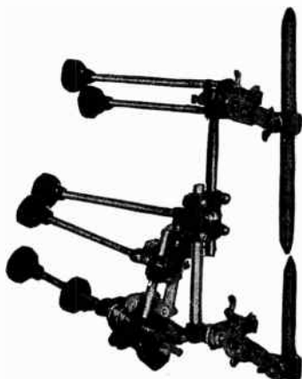
FIG. 3,878. Powers' arc lamp. Carrying capacity 100 amperes. All adjustments are accomplished from the outside of the lamp house. Carbon range from \frac{3}{8} " to \frac{1}{4} " in diameter, 6" length for lower and 12" length for upper carbon. The carbon may be placed at any angle desired, and can be moved independently of each other, forward, backward and sideways, or the whole lamp can be swung forward or backward, laterally, and up and down.
