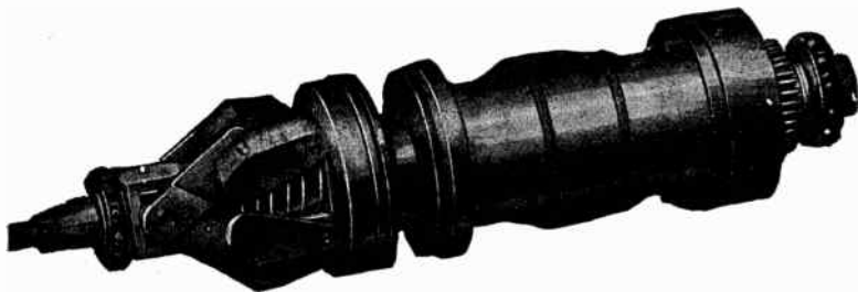
FIG. 3,981. —Automatic spark advance mechanism and armature of Eisemann magneto. The automatic advance is accomplished by the action of centrifugal force on a pair of weight attached at one end to a sleeve through which runs the shaft of the magneto, and hinged at the other end of the armature. Along the armature shaft, run two helicoidal ridges which engage with similarly shaped splines in the sleeve. In operation , the rotation of the armature causes the weights to spread and exert a longitudinal pull on the sleeve which in turn changes the position of the armature with reference to the pole pieces. Thus, the moment of greatest induction is advanced or retarded and with it the break in the primary circuit, for the segments (or cams) which left the circuit breaker and cause the break in the primary circuit are fixed in the correct position and thus the break occurs only at the moment when the current in the winding is strongest. On other magnetos it is the segments or cams that are moved forward or back as the case may be. To apply the automatic control principle to any engine, there have been produced spindles of varying pitches; spindles that will give 19, 25, 38, 45 and 60 degrees advance. For use in connection with these spindles, there are sixteen different springs. With these parts, in connection with the governor mechanism, 160 advance curves can be produced. By varying the length of the stop on the bronze nut, more may be obtained. Many engines require a great deal of advance, others will not permit of more than 20 to 25 degrees. It is necessary to take into consideration the size and shape of the combustion chamber, the compression, the position of the spark plugs and the speed of the motor. It is also universally acknowledged that an engine of high compression will give a quicker burning mixture and will not require, or in some cases, stand, as early a spark as one of lower compression.
