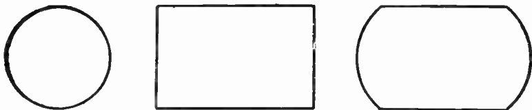
Figs. 3,882 to 3,884. —Various film perforations. These are called: fig. 3,882, round; fig. 3,883, square; fig. 3,884, barrel. The square and barrel holes seem to be more durable than the round hole. The shape of the holes should correspond to the shape of the sprocket teeth. A standard perforation is four pairs of holes per picture, each hole being approximately \frac{1}{16} \times \frac{3}{32} , spaced along the edges of the film \frac{1}{16} inch apart, making four holes at each edge for a \frac{3}{4} inch motion picture image.
