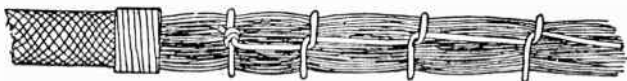
Fig. 2,972.—Manner of lacing a telephone cable. The insulated wires are held in position or laced together by a linen thread saturated with melted crude beeswax, wound around them and tied by slip knots at those points where the wires are taken for connections and bent out.
