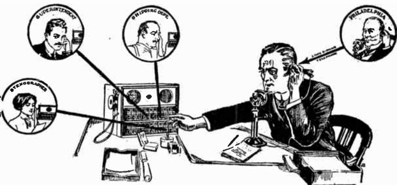
FIG. 3,045.—How the dictograph system is used in business; view showing master station dictograph and several substation dictographs, also long distance telephone. If a telephone call comes to an office manager and he desires information from his employees he talks to them as he would if they were in his presence. By placing his hand over the telephone mouthpiece, he can shield his voice from the telephone.
