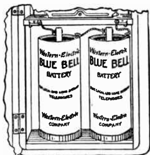
FIG. 2,996.—Installing a magneto set: 3. Connecting the dry cells. For ordinary service two cells suffice, however in the case of long toll connections three cells are recommended. To connect two cells, take one of the loose cords furnished with the set and connect one end to the short outside or zinc terminal, and the other to the long inside or carbon terminal. Place the cells in the lower part of the set and connect the ends of the cords hanging from the terminals on the generator shelf, one to the long part of the first cell, and the other to the short part of the cell.
