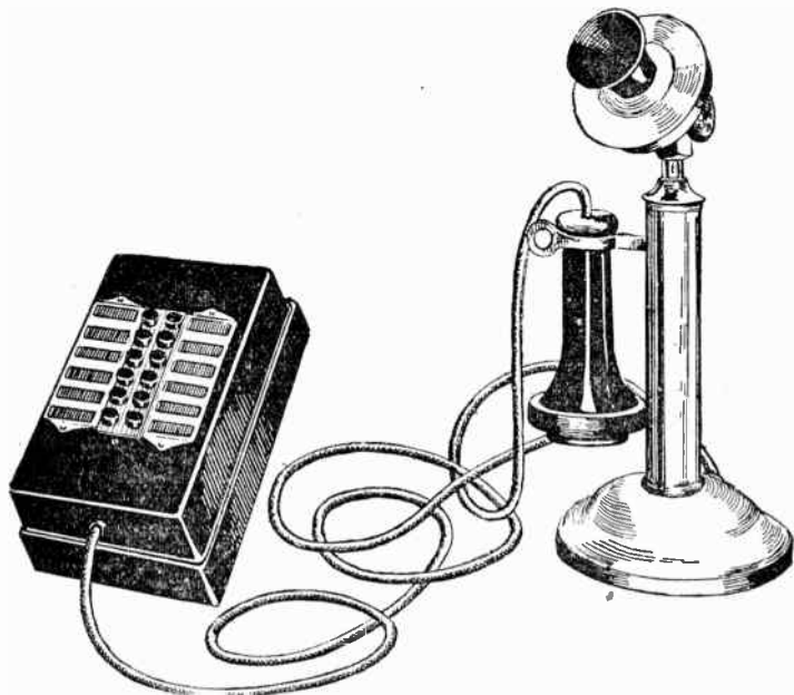
FIG. 2,973. —Western Electric automatic intercommunicating telephone set. This type of instrument is for general use where a high grade of intercommunication is desired. There can be as many stations in the system as there are connected station buttons on the interphone box connecting set. Four additional buttons are connected with the others where the system is used for intercommunicating residence service and connected to a telephone central line. One of these is marked "ring," another "answer," another "transfer," and another "central," depressing any one except "ring" cuts out and automatically restores any other that may be depressed. The "ring" button does not stay depressed like the others. The system permits of any station calling any other and is non-interfering. Several conversations may be carried on at one time between several stations.
