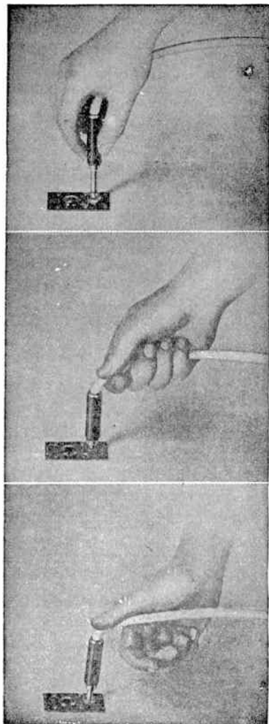
Figs. 3,032 to 3,034.—Removing and inserting plugs. Fig. 3,032 shows incorrect method of inserting a plug; fig. 3,033, incorrect method of removing, and fig. 3,034 correct method of removing and inserting.
