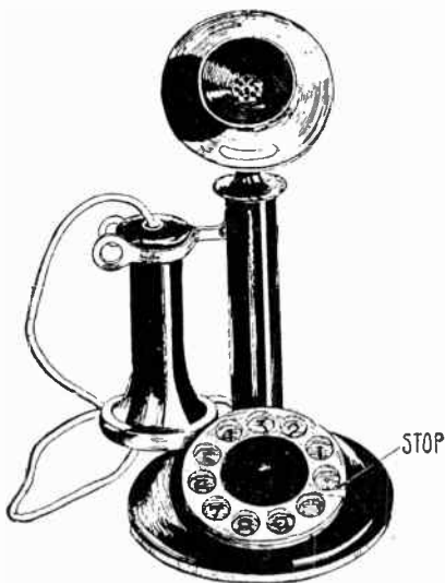
FIG. 2,967.—Automatic selector telephone desk stand with the dial at the base of the instrument. By inserting the finger in the dial at the desired number and revolving it until the stop holds it, electric impulses are sent out through the desk stand cords which register corresponding numbers at the automatic central office. The dial is numbered from 1 to 9, then follows the cipher and "long distance."
