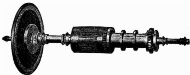
Fig. 2,795. —Rotor of Westinghouse type T turbine dynamo set. The dynamo is of the commutating pole type either shunt or compound wound. The turbine is of the single wheel impulse type. The wheel is mounted directly on the end of the shaft as shown. Steam is used two or more times on the wheel to secure efficiency. A fly ball governor is provided with weights hung on hardened steel knife edges. In case of over speeding, an automatic safety stop throttle valve is tapped shutting off the steam supply. This type of turbine dynamo set is especially applicable for exciter service in modern, superheated steam generating stations where the steam pressure exceeds 125 pounds. Westinghouse Type T turbines operate directly (that is, without a reducing valve) on pressures up to 200 pounds per square inch with steam superheated to 150 degrees Fahrenheit.
