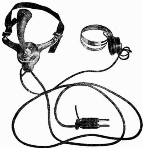
FIG. 2,945. —Operator's equipment showing receiver transmitter cut in plug, etc. The breast plate transmitter equipment is shown with cords connecting it to a cut in plug and a head receiver. The horn shaped mouthpiece is made of hard rubber and can be unscrewed and removed. The breast transmitter is held in place by a cloth neck band, the receiver by a head receiver band and the plug is inserted in spring jacks which are connected with the operator's set.
