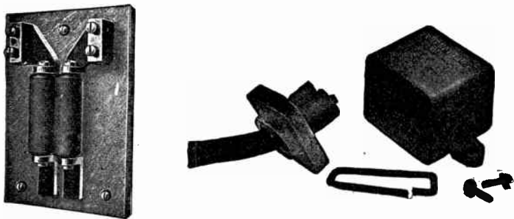
Figs. 2,359 to 2,364. —Westinghouse safety spark gaps. Fig. 2,359, indoor type; figs. 2,360 to 2,364, outdoor type. It is well known that with transformers, operating on high voltage lines and having large ratios of transformation, there may occur, on the low tension side, momentary voltages to ground greatly in excess of the normal. These momentary increases in voltage between the low tension circuits and ground are commonly called "static disturbances." In general they are the result of a change in the static balance of the high tension side and its connecting circuits. Unless certain precautions are taken, such a static disturbance on the low tension side may cause serious stresses in the secondary insulation of a transformer with a high ratio of transformation. This induced static voltage is independent of the ratio of transformation. The static stresses are more serious in a high ratio transformer simply because the insulation of its secondary is less able to withstand them. A method of relieving this disturbance is to connect a discharge spark gap between some point of the low tension side of the transformer to be protected (a middle or neutral point, if one be available) and the ground. The spark gap opening is such that any voltage very much in excess of the maximum normal will cause a discharge to ground, and thus the low tension side is practically tied to ground during such disturbance, while at other times it is ungrounded. The Underwriters recommend the grounding of the neutral point of low tension circuits when the conditions are such that the maximum normal voltage between the point connected and ground will not exceed 250 volts. The rule allows one side of a 250 volt circuit or the middle point of a 550 volt circuit to be grounded. The spark gaps shown above are designed for use on transformer secondary circuits and for protecting individual series arc lamps. These spark gaps are single pole, and consist of two cylinders of non-arcing metal with an air gap between. One of the cylinders is connected to the ground, the other to the line.
