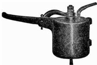
FIG. 2.271.—General Electric shunt trip attachment. The shunt trip attachment has been designed to provide for conditions under which the low voltage attachment cannot be successfully applied. It resembles the low voltage attachment in construction, but differs in that it trips the circuit breaker when energized. The shunt trip should be allowed to remain only momentarily in circuit; hence it should be so connected that the opening of the circuit breaker immediately disconnects it from the circuit. Whenever it is impossible to connect the shunt trip in this manner, the circuit opening auxiliary switch should be used in connection with it.
