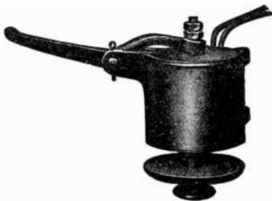
FIG. 2.272.—General Electric low voltage trip attachment for circuit breakers. This low voltage trip is designed to operate the circuit breaker when the line voltage drops to approximately 50 per cent or less of the normal voltage. It should be noted that the coil is always in circuit, as is the case with the overload and underload coils, and that it operates with the releasing of its armature. It is always necessary to use a fixed amount of resistance (depending upon the voltage of the system) in series with the low voltage release. The low voltage release performs the functions of a shunt trip coil when used in conjunction with a push button, auxiliary switch or speed limiting device, and is generally preferred to the shunt trip attachment.
