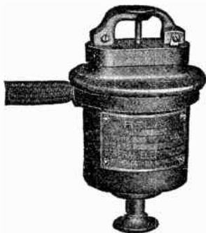
FIG. 2,301.—Alternating current low voltage circuit closing low voltage relay, for 600 volts or less. The contacts are similar to those of the circuit closing overload type except that they are inverted. As long as the pressure is normal the contact cone is held above the contacts. When the pressure falls below one half normal, the cone and plunger rod drop and close the contact. This relay does not pick up its own plunger. The plunger rod is pushed up by hand after the pressure circuit is established. Low voltage relays are generally used in connection with a low voltage release or shunt trip coil on an oil switch or a circuit breaker. They are used in connection with motor booster sets to prevent a disastrous speed of the booster which might result from the loss of alternating current power. They are also sometimes used for indicating purposes.
