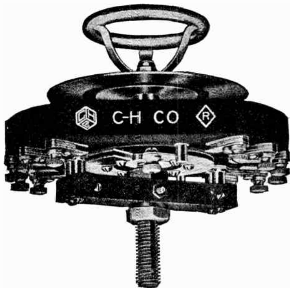
FIG. 2,669.—Crouse-Hinds radial ammeter switch, arranged for mounting directly on the switchboard. It is designed for use with external shunt ammeters of any make or capacity, and in conjunction with the required number of shunts, makes possible the taking of current readings of a corresponding number of circuits by means of one ammeter. The wiring diagram is shown in fig. 2,670.
