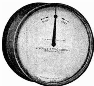
Fig. 2,571. —General Electric synchronism indicator. The synchronism indicator is a motor whose field is supplied with single phase current from one of the machines to be synchronized, and its armature from the other. The armature carries two inductance coils placed at a large angle, one supplied through a resistance, the other through an inductance. This arrangement generates a rotating field in the armature, while the stationary field is alternating. The armature tends to assume a position where the two fields coincide when the alternating field passes through its maximum; hence, the armature and pointer move forward or backward at a rate corresponding to the difference of frequency, and the position when stationary depends on the phase relation. When the machines are running at the same frequency and in phase the pointer is stationary at the marked point. In construction, it is like a small, two phase, bipolar synchronous motor, the field being supplied with alternating instead of direct current. The armature is mounted in ball bearings in order to make it sufficiently sensitive and smooth in operating. The armature coils are not exactly 90 degrees apart, since it is not possible to get the current in the two coils exactly in quadrature without introducing condensers on other complicated construction. Standard ratings are for 110 and 220 volt circuits. Synchronism indicators should be ordered for the frequency of the circuit on which they are to be operated, although the instruments may be used on circuits varying 10 per cent to 15 per cent from the normal. The words "Fast" and "Slow" on the dial indicate that the frequency on binding posts E and F is respectively higher or lower than that on A and B; or, in other words, clockwise rotation of the pointer means that the incoming machine is running at too high speed, counter clockwise rotation indicating too low speed.
