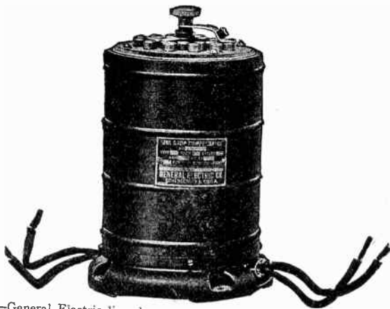
FIG. 2,460. —General Electric line drop compensator. This compensator contains besides resistance and inductance, a current transformer, the secondary of the transformer being connected in series with the resistance and inductance; the primary of the contained current transformer is connected to an external current transformer. The reactance and resistance are both so wound that any proportion of the winding can be cut in or out of the voltmeter circuit. Both elements have 12 points of adjustment of one volt each, giving a total combined drop at maximum setting of about 17 volts.
