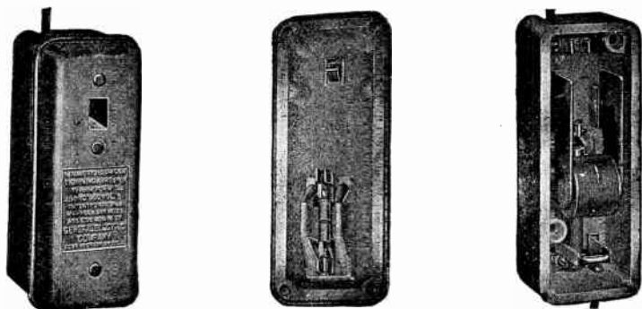
FIGS. 2,402 to 2,404. —General Electric magnetic blow out arrester for use on railways. It consists of an adjustable spark gap in series with a resistance. Part of the resistance is in shunt with a blow out coil, between the poles of which is the spark gap. The parts are mounted in a strong, porcelain box, which, for car and pole use, is in turn mounted in a substantial asbestos lined, wooden box. In operation, when the lightning pressure comes on the line, it causes the spark gap to break down and a discharge occurs through the gap and the resistance rod to ground. Part of the current shunts through the blow out coil producing a strong magnetic field across the spark gap. The magnetic field blows out the discharge arc and restores normal conditions. The resistance is only 60 ohms (for 500 volt rating work), and the spark gap only one-fortieth of an inch (.025 in.).
