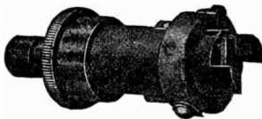
FIG. 2,274.—General Electric circuit closing auxiliary switch . This switch closes when the circuit breaker opens, and may be used to announce the automatic opening of the circuit breaker through the means of an indicating lamp or an alarm bell. It is often necessary to arrange one circuit breaker so that, in opening, it will trip others. This may be accomplished by using a circuit closing auxiliary switch in connection with a low voltage or shunt trip attachment on the circuit breakers to be tripped. The construction of this type of switch is such that it may be opened by hand after the circuit breaker opens, but it is automatically reset when the circuit breaker is closed.
