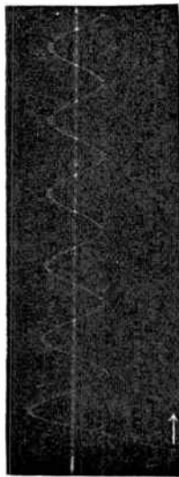
FIG. 2,632.—Mazda (tungsten) lamp, showing rapid decrease to normal current as filament heats up. 25 cycles.
