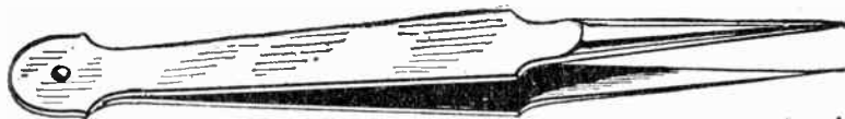
FIG. 4,471. —Brazing the joint of a pair of tweezers. The surfaces to be brazed are cleaned some of the spelter applied to each surface, and the pieces tied together with a fine iron wire and heated sufficiently to melt the spelter. The heat may be applied with a blow pipe or by holding the pieces in a pair of hot tongs. When the spelter is melted the piece is cooled and the iron wire is taken off. When the pieces are clamped in hot tongs, the iron wire is sometimes omitted, the pieces being placed in their proper relation and the tongs depended on to keep them there, or stops may be arranged to determine the location of the pieces.
