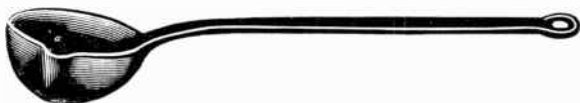
FIG. 4,426.—Ladle for removing solder from soldering pot and for pouring same in making wipe joints, etc.
