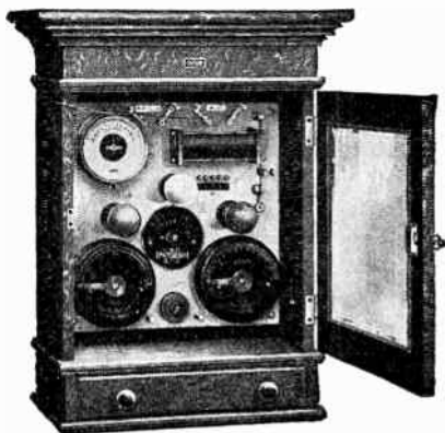
FIG. 4.645. —McIntosh type 12 aseptically porcelainized plate. Direct current operation. When the plate is employed with direct current lighting circuit, the galvanic and faradic circuits of the plate are supplied by the direct current; while a motor generator must be employed to transform the direct current to an alternating current to properly energize the transformer for cautery and sinusoidal currents. In this manner each circuit of the plate is supplied with its appropriate form of energy. Battery equipment. With a battery of 50 dry cells and a motor generator the same results can be had as with the direct lighting current, the cells being good for 100 brief cautery operations and several hundred galvanic, faradic and sinusoidal applications. Dry cells, however, constitute an expensive current service. Alternating current installation. With the alternating current the rectifier with pressure equalizer is necessary to transform the alternating current to a direct current in order to operate the galvanic and faradic circuits, while the alternating current in its original form is employed with the transformer for cautery and sinusoidal currents. The dial current selector. With one turn of the knob all connections for any given modality are instantly made and the current is ready for use. Eleven distinct modalities are plainly indicated on the dial. When the knob is turned "off", the current is completely cut off from all circuits of the plate. The rheostat. This consists of a solid block of porcelain, wound with high grade resistance wire, with a traveling contact which increases or diminishes the current strength imperceptibly controlling the galvanic, faradic and sinusoidal currents. The volt scale shows the voltage of galvanic current used. Monomotive rheotome. This is an interrupter, which may be used to interrupt either the galvanic, faradic or sinusoidal currents; being especially valuable with the former in muscular diagnosis. It is wound up as a clock by means of the key accompanying the outfit, and, as its name indicates, requires but one motion to start mechanism, select frequency, and close circuit. The faradic coil. This is a secondary coil with a primary winding of 230 feet of No. 20, a rather coarse wire; and a secondary of 1,300 feet of No. 30, a comparatively fine wire, thus affording a comprehensive range of induced currents. The slowly interrupted faradic currents are secured with the monomotive rheotome, varying from 20 to 400 per minute. The transformer. This transforms alternating current of 110 volts, 1\frac{1}{2} amperes, to a cautery current (which is also an alternating current) of 4 volts, 35 amperes, sufficient for all ordinary knives, under perfect control of operator. The sinusoidal current obtained from the transformer is "earth free," having no "ground" connection, and, if desired, may be used in bath tub application, something unattainable with the ordinary wall plate on account of the average bath tub being grounded by the waste pipe connection. This feature is of especial value in a sanitarium. Milli-ampere meter. The meter has two scales, one in black figures reading 0-400, suitable for recording heavy dosages, which is placed in service by inserting the hard rubber plug in the socket marked "B;" and one in red figures reading 0-20, adapted to measuring lighter currents, which is in effect when the hard rubber plug is inserted in socket marked "R." The meter reads to right or left according to position of pole changer. Before using meter, the knob on scale pan may be adjusted so that the needle rests exactly at zero.
