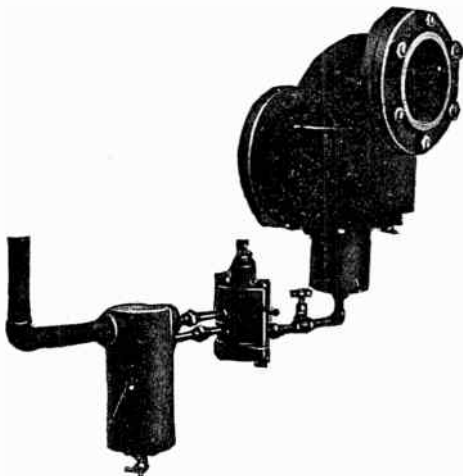
FIG. 4.381.—Ingersoll-Rand Imperial unloader. It operates by closing the air intake, and automatically regulates the compressor, maintaining the line pressure within a satisfactory range. It consists of a valve on the compressor intake pipe, normally held open by its own weight. When receiver pressure rises above normal this pressure is communicated through a small pipe from the regulating valve, acting to close the valve in the intake pipe, thus shutting off the air supply. The regulating valve can be adjusted for any working pressure by means of a spring adjusting screw.
