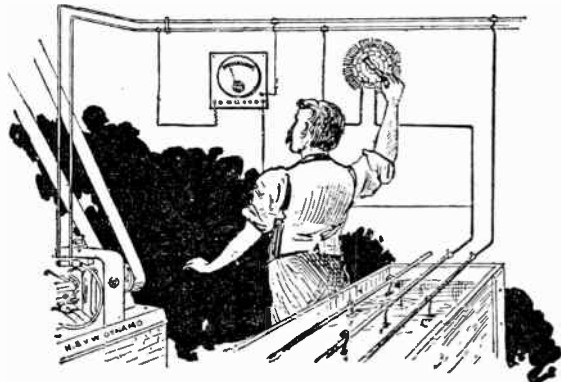
FIG. 4,557.—Connections and manipulation of rheostat on large copper, brass, and bronze solutions where variations of voltage are necessary to secure different colors.
