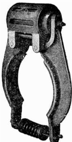
FIG. 4,186.—Detail of Kaestner and Hecht electric brakes. In operation , the brake is mechanically closed by the spring shown at the lower end, and electrically released by the solenoid at the top.
