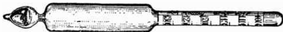
FIG. 4,623.—Acid hydrometer for testing the density of the electrolyte of acid electrolytic interrupters. It is important to have the specific gravity of the acid as follows: For a 110 volt current, 1,220; for a 220 volt current 1,070 Baume. The specific gravity can be approximately obtained by mixing ingredients according to the formula sent with the interrupter, but as this will vary from the evaporation of the water, it is advisable to use a hydrometer to determine when ( distilled ) water must be added, or when making a new solution. It should be noted that the reading of a hydrometer varies with the temperature, accordingly the reading must be corrected. Some hydrometers have a thermometer and correction scale in the neck.
