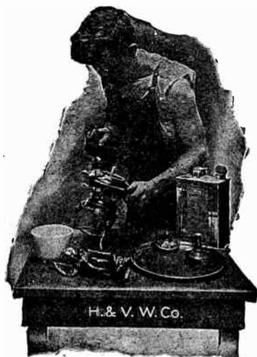
FIG. 4,575. —Method of applying lacquers. Instructions: Use a glass tumbler or porcelain cup as a container. Apply a flowing coat with a soft brush. A stiff brush will cause foaming or small air bubbles, and will require a heavier body lacquer. Prepare the work the same as for plating. It must be absolutely clean and free from grease or moisture. It requires only the smallest amount of moisture to ruin the work. Use the lacquer as thin as possible without showing iridescent colors. Dry in a temperature of 100° Fahr., if possible, using a thermometer. Brush lacquers will dry in the ordinary temperature, but baking improves the finish. Iridescent colors are in most cases caused by the lacquer being too thin, or by carelessness in removing the polishing composition or rouge from the work. Iridescent colors will often disappear when the article is given a second coating of lacquer after the first has dried. When the body becomes too heavy it needs thinner. Be sure to use only a thinner of the same grade as the lacquer.
