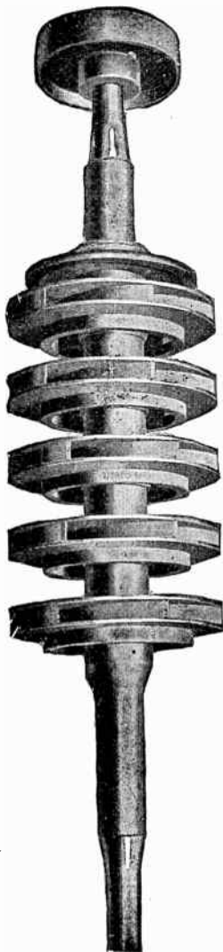
FIG. 4,315.—Rotating element or impellers of Allis-Chalmers five stage centrifugal pump showing runners and balancing disc.
