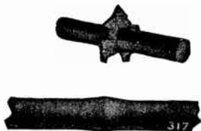
Figs. 4,517 and 4,518. —Flash weld, and upset weld. A flash weld is generally used on stock that is wide and thin; where it is rectangular in shape, and where it is not possible to have the welding faces cut square and true. Also in welding tubing to forgings, or tubing to tubing. In all cases where a small amount of stock is to be taken up in welds, or when it is desired to shear or grind off the fin, a flash weld is made. Upset welding is used in all cases where the weld is to be hammered, using the heat generated in the welding. Also for small rods or rings where it is not necessary to have a uniform thickness of stock. On brass or copper a flash weld is made. Three times the diameter of stock between the dies should be allowed on brass and four times on copper, but only once the diameter of stock is actually taken up in the weld.
