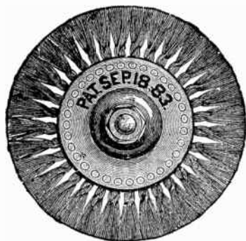
FIGS. 4,568 to 4,571.—Hanson and Van Winkle swing type, circular steel wire, casting brush. The steel wires are twisted in knots and the knots are hung on rods around the hub, as shown in fig. 4,571, so that they will turn around the rods if the work be held too close to the brush wheel. In using the brush the work should be held so as to be just in contact with the ends of the wires. The brush shown is about 15 inches in diameter, and should not be run much faster than at the rate of 1,000 revolutions per minute. If the brush be run too fast, or if the work be held too close, the wires will become crystallized and soon break off. After the brush has been run for a while, the ends of the wires will become bent and drag over the surface of the work; the brush should then be taken off the spindle, turned around, and replaced with the hub next to the collar on the spindle, so that the wire ends will again strike the surface of the work. When the wires are worn out a new set of knot can be readily substituted for the old set by unscrewing the nut N and taking off the hub plate P.
