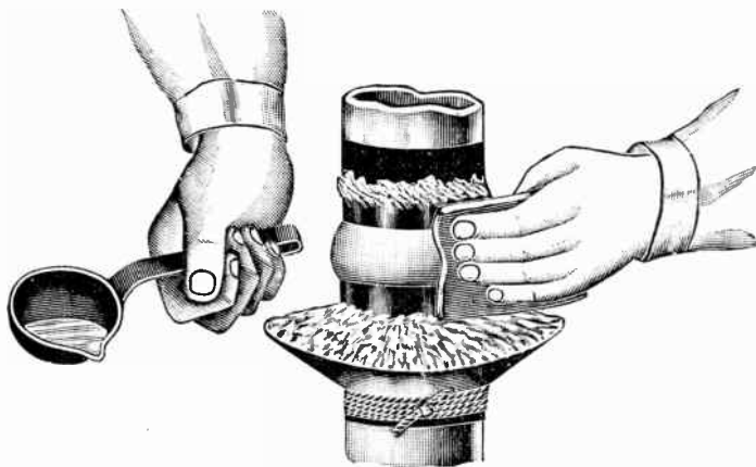
FIG. 4,435.—Method of wiping a vertical joint. A small piece of cardboard cut open is placed under the joint to catch excess solder, or as shown, a lead flange cut open is placed around the pipe and held in place by twine.
