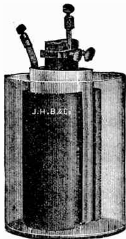
FIG. 51. —The Bunsen cell. This is a two fluid cell and has a bar of carbon immersed in strong nitric acid contained in a porous cup. This cup is then placed in another vessel, containing dilute sulphuric acid, and immersed in the same liquid, is a hollow cylindrical plate of zinc, which nearly surrounds the porous cup. The hydrogen, starting at the zinc, traverses by composition and recombination, the sulphuric acid; it then passes through the porous partition, and enters into chemical action with the nitric acid, so that none of it reaches the carbon. Water is produced by this action, which in time dilutes the acid, and orange colored poisonous fumes of nitric oxide rise from the battery. If the nitric acid first be saturated with nitrate of ammonia, the acid will last longer and the fumes be prevented. Strong sulphuric acid cannot be used in any battery; one part of sulphuric acid is generally added to 12 parts by weight, or 20 by volume, of water. Grove used a strip of platinum instead of carbon in his cell. A solution of bichromate of potassium is frequently substituted for the nitric acid in the porous cup, thereby avoiding disagreeable fumes. Bunsen's and Grove's cells produce powerful and constant currents, and are well adapted for experiments, but they require frequent attention, and are expensive, so that they are little used for work of long duration. The electromotive force of these cells is from 1.75 to 9.51 volts.
