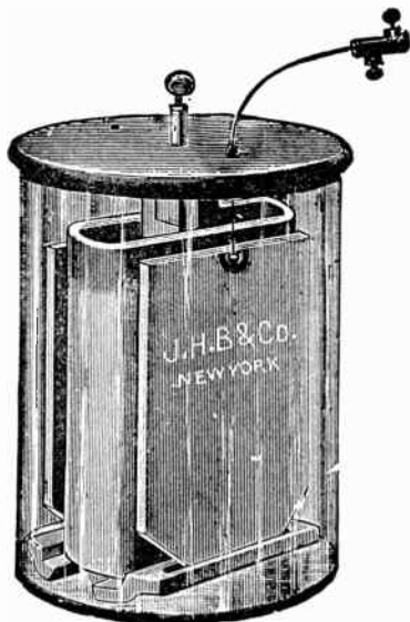
FIG. 55.—Wheelock cell; the elements are carbon and zinc. To set up, place the grid in the bottom of the jar and fill its two troughs each about half full of mercury. Place the porous cell in position on the grid so that it sits perfectly upright, resting in the recess of the latter. The zincs stand with lower ends resting in mercury in the troughs of the grid. Into the porous cell, to a height of only two thirds full, pour solution consisting of equal parts water and sulphuric acid, by measure. Add to this \frac{1}{2} pound nitrate soda, 1 ounce chromic acid. This solution may be made up in the above proportion and kept in covered receptacle in any desired quantity, ready for use. In the outer jar for 6 x 8 size, 2\frac{1}{2} pints of water, and \frac{1}{2} gill sulphuric acid, 1 part sulphuric acid to 20 parts water, or as much sulphuric acid as it will take without boiling. When a charge becomes exhausted it may be renewed by adding sulphuric acid and salts in the proportions given above, after drawing out with syringe enough of the old solutions to make room for the additions, but the best action is obtained with entirely new solutions. Zincs must be kept thoroughly amalgamated by keeping a good supply of mercury in the troughs.
