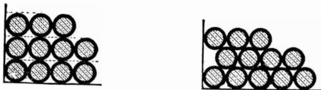
Figs. 242 and 243.—Square and hexagonal order of "bedding." The term bedding is an expression used to indicate the relation between the cross sectional area of the winding when wound square, as in fig. 242, and when wound in some other way, as in fig. 243. In the square order of bedding, the degree of bedding equals zero.
