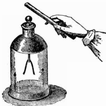
FIG. 11.—Gold leaf electroscope; it consists of two strips of gold foil suspended from a brass rod within a glass jar. Used to detect the presence and sign of an electric charge.
