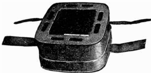
FIG. 246.—Port Wayne compound wound rectangular ventilated spool field coil. The series and shunt coils are wound side by side, ventilating passages being provided lengthwise through each coil and between the shunt and series coils as shown.
