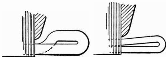
FIGS. 375 and 376.—Single layer and double layer barrel winding. Barrel winding is a method of arranging the ends of armature coils as they pass from one pole to the next, in which, instead of using involute or butterfly connections, V-shaped end connections are used which lie on a cylindrical surface, which is a continuation of the armature surface. The coil ends must of necessity be arranged in two layers, but the method may be used for either one or two coils per slot, the difference in arrangement for these is here illustrated.
