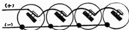
FIG. 73.—Diagram of a multiple or parallel connection. When connected in this manner the voltage of the battery is the same as that of a single cell, but the current is equal to the amperage of a single cell multiplied by the number of cells. Thus with 1\frac{1}{2} volt 15 ampere dry cells, the combination or battery connected as shown would give 4 \times 15 = 60 amperes at a pressure of 1\frac{1}{2} volts.
