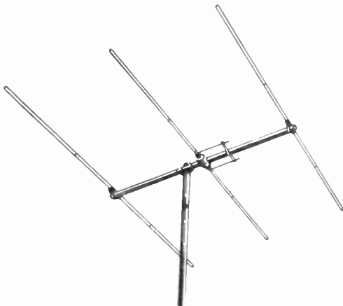
Fig. 14. A typical beam antenna used for two-way radiocommunications.
