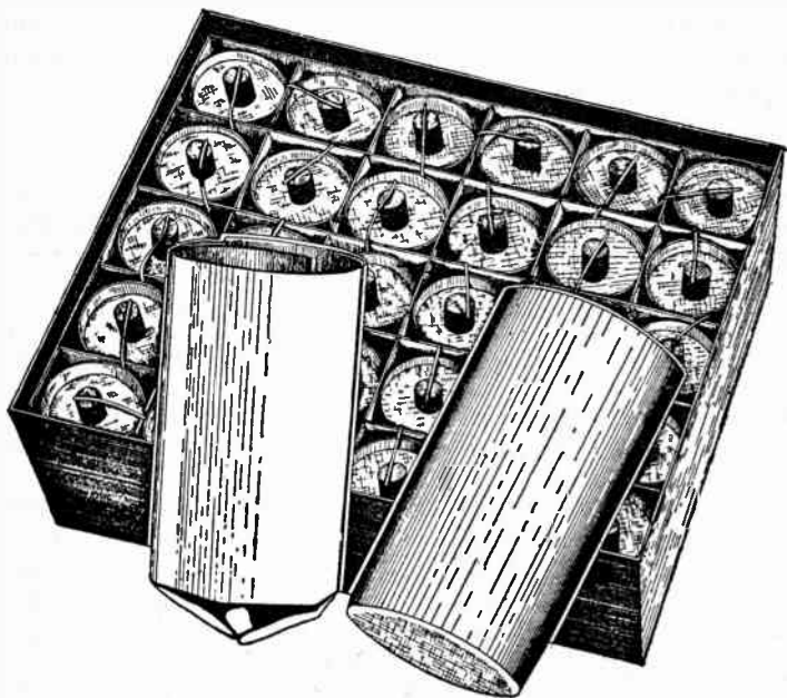
FIG. 5.—Klearstone dry battery with top removed showing what the inside of a 45 volt B battery looks like. The illustration also shows at the right the one piece seamless zinc cup, and at the left the paper insulator and filter which fits inside it.
