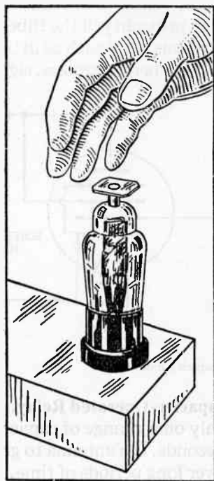
FIG. 37.—If a sensitive current indicator be connected as shown in fig. 36, the meter will show the current change due to the capacity effect, if a hand be placed in proximity to the antenna.
