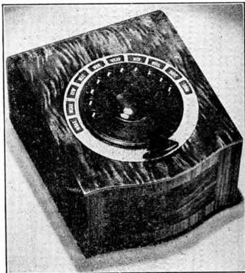
FIGS. 10 and 11—Fig. 10 shows circuit diagram of the portable control box. Impulses sent out from the box are picked up by the five tube unit (fig. 12) and amplified to the proper degree to actuate the tuning mechanism shown in fig. 13. All control boxes are adjusted to use one of the five frequencies specified above.
