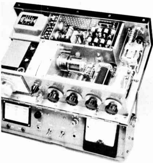
Fig. 19-21—The 65-watt mobile transmitter has a Nuvistor v.f.o., a 6146 output stage and transistors in the modulator and power supply. In this view the sheet-metal top and sides have been removed to show the arrangement of parts. The panel carrying the meter and switches (see Fig. 19-23) is recessed in a 3\frac{1}{2} high \times 2\frac{3}{4} deep by 14-inch box; the box is hinged and folds up when the transmitter is not in use. Major chassis is built from \frac{3}{8} -inch wide by \frac{1}{8} -inch thick aluminum angle and a 9 \times 14 -inch sheet of aluminum. A ventilation hole covered with cane metal is partially visible below the 6146 (center).
