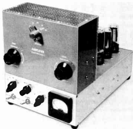
Fig. 6-51—Front view of the 6146 all-purpose amplifier. The upper panel is part of an 8 × 6 × 3½-inch Minibox (Bud CU-2109); the ventilated shielding of Reynolds Aluminium cane metal is fastened to the Minibox and base with sheet-metal screws.
