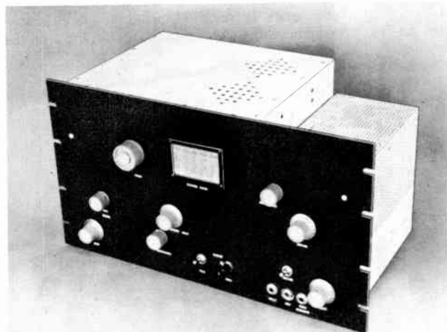
Fig. 17-23—The high-power 2-meter rig, with shielding enclosures in place. The small unit at the right houses the tripler and driver stages.
