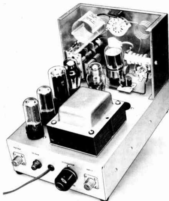
Fig. 6-52—Rear view of the 90-watt all-purpose amplifier with the cane-metal cover removed. One voltage-regulator tube has been removed from its socket (right edge of transformer) to allow the neutralizing capacitor and plate blocking capacitor to be seen. The plate r.f. choke (RFC 3 in Fig. 6-49) is mounted on one side wall, and the load capacitor and safety choke (C 1 and RFC 1 in Fig. 6-53) are mounted on the far side wall.
