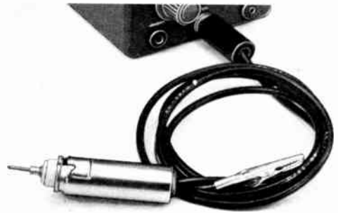
Fig. 21-32—The r.f. probe is used in conjunction with a vacuum-tube voltmeter. The case of the probe is constructed from a 7-pin ceramic tube socket and a 2¼-inch tube shield. A half-inch grommet at the top of the tube shield prevents the output lead of the probe from chafing. The flexible copper-braid grounding lead and alligator clip provide a low-inductance return path from the test circuit. The d.c. output of the probe goes to the phone plug, which plugs into the d.c. input jack of the v.t.v.m.
