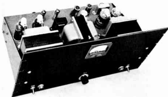
Fig. 8-23—Class-AB 1 modulator using 6146s, complete with speech amplifier and power supply. The relay-rack panel is 10½-inches high. Plate- and filament-supply primary switches, each with its own pilot lamp, are near the lower edge of the panel. The gain control is at lower center. Along the front of the chassis, just behind the panel, are the plate power transformer, filter choke, and modulation transformer, going from left to right. The tubes at the left are the 816 rectifiers, with the 6146s at the right. Along the rear edge are the two voltage-regulator tubes, the 12AX7 and 6C4 speech amplifier tubes, and the inter-stage audio transformer, T_1 .
