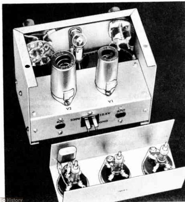
Fig. 19-7—Homemade L-shaped chassis, mounted on small brackets fastened to the side walls of the converter housing, is 4\frac{15}{16} inches long, 2 inches wide and 1\frac{1}{2} inches deep. V_1 is mounted on the chassis to the right of V_2 as seen in this rear view. J_1 , J_3 and J_2 are in line in that order from right to left across the rear wall of the chassis. An interior view of a coil compartment is shown in the foreground. Terminals of the coils are soldered directly to the socket terminals. Notice that the crystal for the oscillator is mounted adjacent to L_4 .
