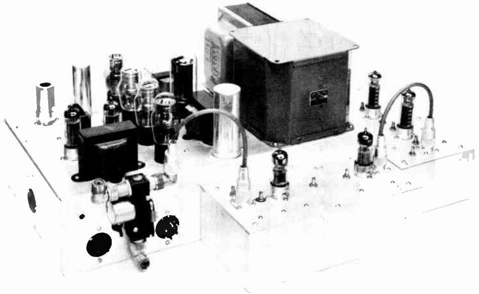
Fig. 17-13—Rear view of the power supply and modulator, with the 144- and 432-Mc. units in place, for 432-Mc. operation. The 432-Mc. unit is in the foreground; its power plug plugs into a socket on the 144-Mc. driver. The six-prong plug to the right of the antenna changeover relay is an outlet for v.f.o. power and control, and the phono jack to the right is J_5 , for receiver output. Socket on the side of the chassis is J_4 , for converter power. The fourth VR tube, visible here but not shown in Fig. 17-14, is for possible use with a receiver/converter power supply.
