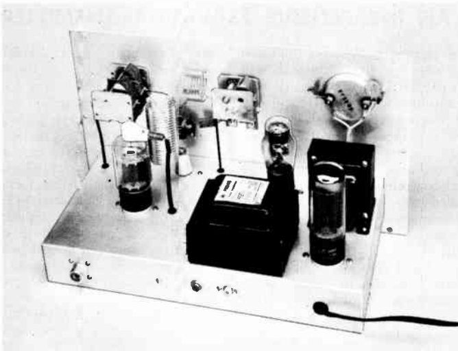
Fig. 6-37—Rear view of the transmitter showing the placement of components above chassis. The loading capacitor, C_5 , is at the left, L_3 is the vertical coil and L_2 the horizontal one. Rubber grommets are used to prevent chafing and to furnish additional insulation on the leads coming from below chassis.
