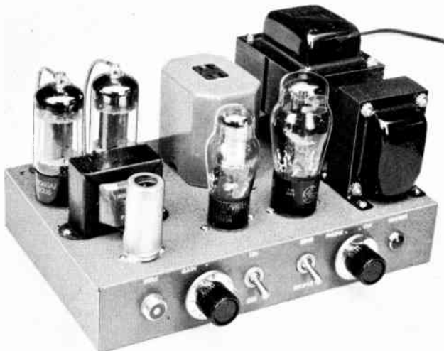
Fig. 8-17—A modulator for transmitters operating at plate inputs up to 50 watts. The speech amplifier and modulator are on the left in this view; power supply components are on the right. The chassis is 7 × 11 × 2 inches.
