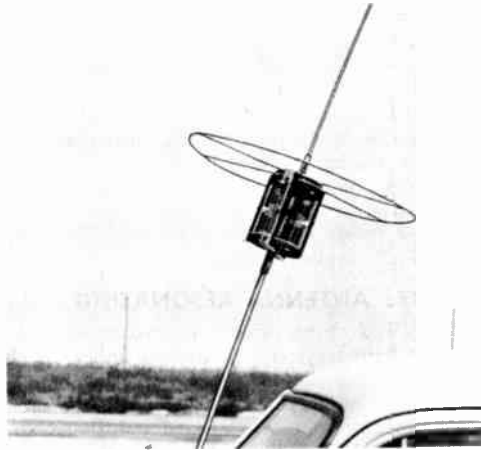
Fig. 19-35—The top-loaded 4-Mc. antenna designed by W6SCX. The loading coil is a B & W transmitting coil. The coil can be tuned by the variable link which is connected in series with the two halves of the coil.
