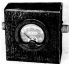
Fig. 21-28—R.f. ammeter mounted for connecting into a coaxial line for measuring power. A "2-inch" instrument will fit into a 2 × 4 × 4 metal box.
