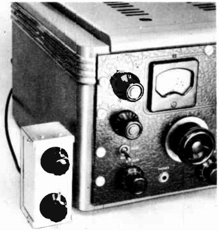
Fig. 5-55—View of the Q multiplier showing its single connecting cable to the receiver. The box can be placed in any convenient spot on or around the receiver.
