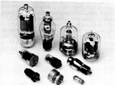
Representative tube types. Transmitting tubes having up to 500-watt capability are shown in the back row. The tube with the top cap in the middle row is a low-power transmitting type. Others are receiving tubes, with the exception of the one in the center foreground which is a v.h.f. transmitting type.
