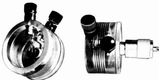
Fig. 21-50 — Balun construction (W2ZE). 150-ohm Twin-Lead may be used for the bifilar winding in place of the ordinary wire shown. Symmetrical construction with tight coupling between the two coils is essential to good performance.
