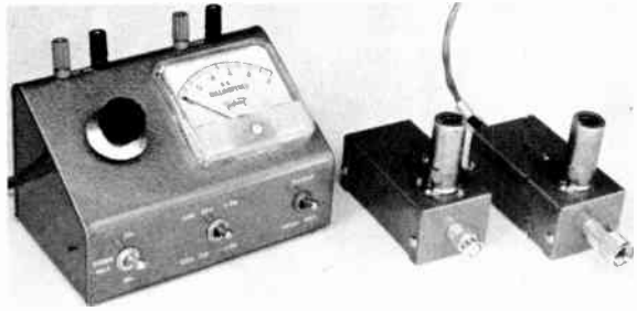
Fig. 21-24—Two diode noise generators and (left) their power supply. Useful generator range is (right) 7 to 90 Mc. and (center) 90 to 450 Mc.
