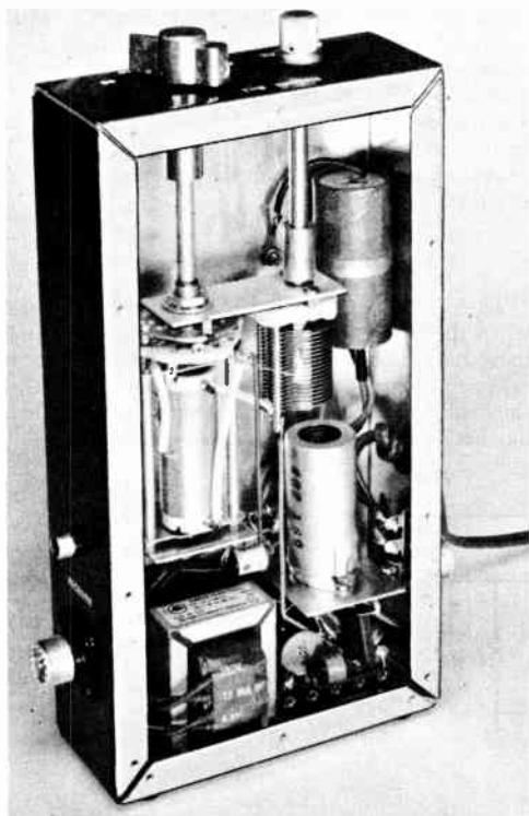
Fig. 22-3—The electronic t.r. switch is built in a 5 \times 9 \times 2\frac{1}{2} -inch chassis. Although two receiver outlets are shown on the near face (a phono jack and a coaxial receptacle), only one is required, depending upon one's choice of cable termination.
