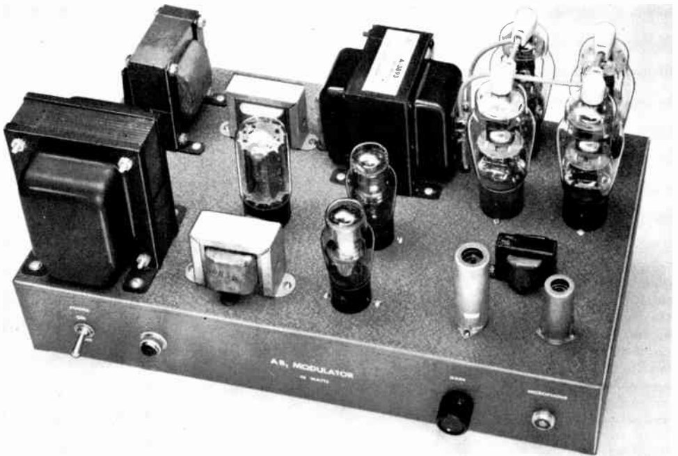
Fig. 8-20—A 50-watt modulator, using four 1625-type tubes in Class AB 1 . With higher plate voltage and a larger modulation transformer, the tubes can deliver up to 140 watts of audio power.
