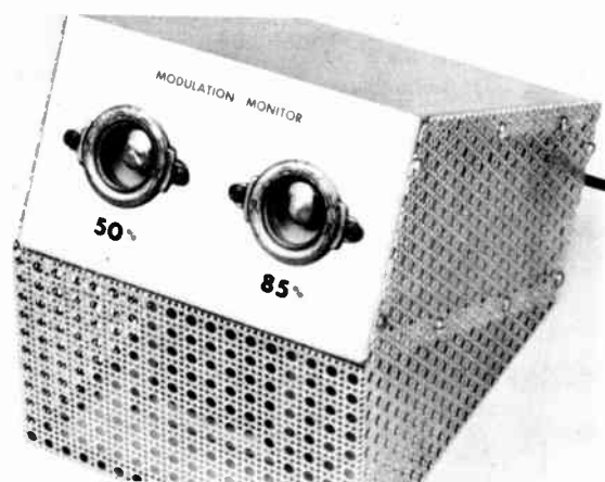
Fig. 11-12—An a.m. modulation indicator using two inexpensive magic eye tubes. It is to be connected to the plate supply and modulation transformer of the plate-modulated transmitter stage. The monitor is built in one half of a Minibox and the entire assembly is supported by a cane-metal housing. Heater transformers hang down from the Minibox, inside the housing.
