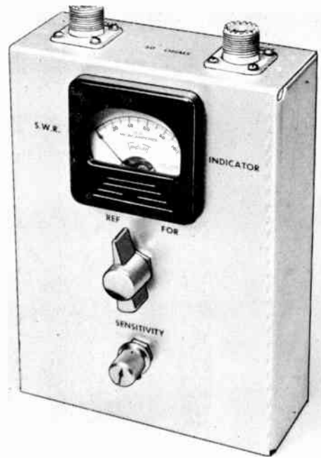
Fig. 13-21—The Monimatch, an s.w.r. monitor that can be left in the line at all times. The unit shown here will handle a kilowatt.
