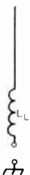
Fig. 19-37 — The capacitive reactance at frequencies lower than the resonant frequency of the whip can be canceled out by adding an equivalent inductive reactance in the form of a loading coil in series with the antenna.
