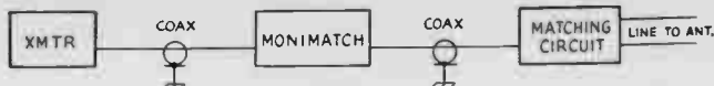
Fig. 13-27— Adjustment setup using the “Monimatch.” This setup applies with any type of matching circuit designed to match a coaxial line from the transmitter.
