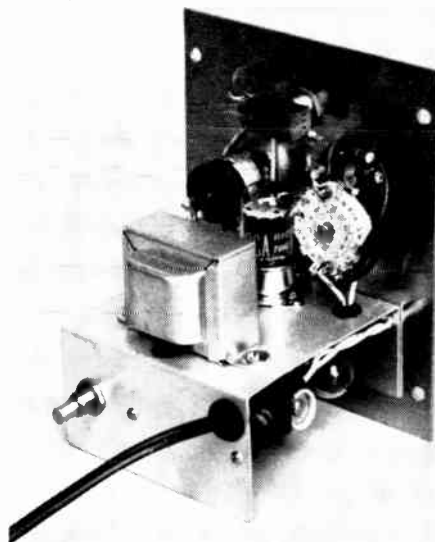
Fig. 21-26 — Inside view of the audio oscillator. The a.c. switch, S_3 , is mounted on the output control at the left on the panel. The ceramic capacitors in the frequency-determining circuits are mounted on the rotary switch, S_1 , at the right. S_2 is above the tube, and T_1 is on the near edge of the chassis, which is a U-shaped piece of aluminum 3\frac{1}{2} inches deep with 1\frac{1}{2} inch lips. R_1 is mounted on the near lip at the left.
