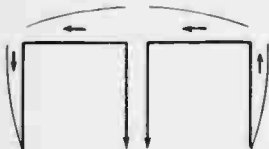
Fig. 14-20 — Folded arrangement for shortened antennas. The total length is a half-wave, not including the feeders. The horizontal part is made as long as convenient and the ends dropped down to make up the required length. The ends may be bent back on themselves like feeders to cancel radiation partially. The horizontal section should be at least a quarter wave long.
