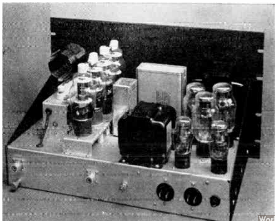
Fig. 11-11 — The power supply occupies the right-hand half of the 17 × 10 × 3-inch chassis and the r.f. section the left-hand half in this view. The power transformer and filter choke is at the edge of the chassis next to the voltage-regulator tubes. The panel is 10½ by 19 inches.
