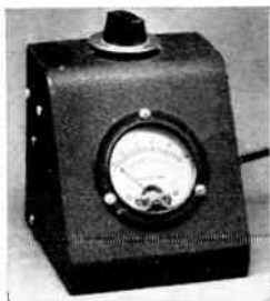
◆ Fig. 21-22—Power supply and milliammeter for the grid-dip meter are contained in a meter case. The control on top is for varying the plate voltage to maintain the grid current in the proper region.
