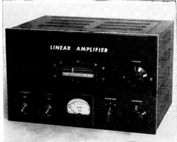
Fig. 11-17 — This linear amplifier uses four parallel-connected tetrodes in a grounded-grid circuit. It can be driven by an s.s.b. exciter capable of 20 watts peak envelope power output. The cabinet is 14½ by 9 by 10 inches deep.
