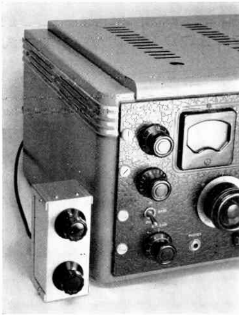
Fig. 5-65 — View of the Q multiplier showing its single connecting cable to the receiver. The box can be placed in any convenient spot on or around the receiver.
