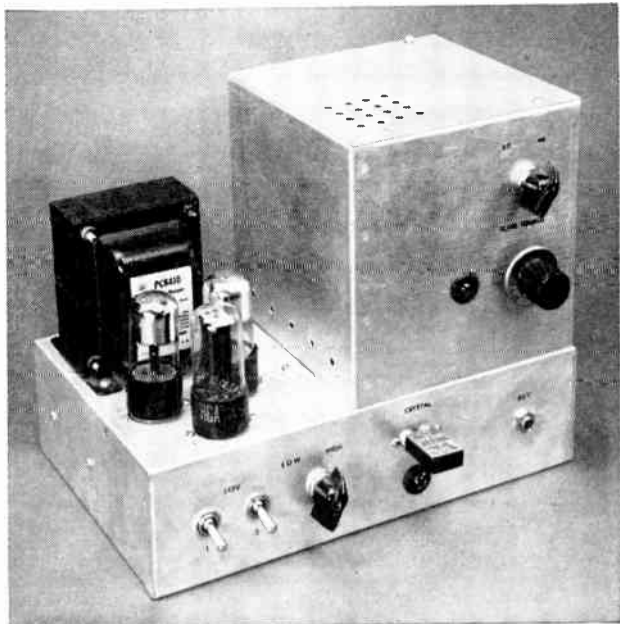
Fig. 6-39 — Pictured is the completed 6146 rig. The plate-current indicator lamp is to the left of the tuning knob. In areas where TVI is likely to be a problem, a metal bottom plate should be used on the chassis in addition to the 6 \times 6 \times 6 aluminum box shown.
