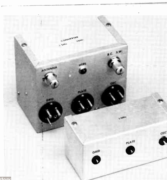
Fig. 19-4. The aluminum case for the converter measures 3 \times 4 \times 5 inches (Bud CA-3005 or Premier AMC-1005). Amphenol type 86-CP4 male jacks mounted on the front of the box mate with MIP 4-prong sockets mounted on the rear of the coil compartment shown in the foreground. Knobs for C_1 and S_1 are to the left and right, respectively, of the pilot lamp. The coil box measures 2\frac{1}{4} \times 2\frac{1}{4} \times 5 inches (Bud CA-3004 or Premier AMC-1004). Slug-adjustment screws for L_2 , L_3 and L_4 protrude through rubber grommets mounted on the front wall of the plug-in coil assembly.
