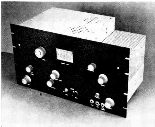
Fig. 17-9 — The high-power 2-meter rig, with shielding enclosures in place. The small unit at the right houses the tripler and driver stages.
