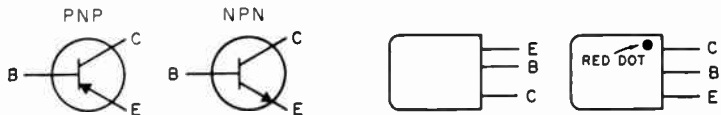
Code for identifying junction transistors. The leads are marked C-collector, B-base and E-emitter.
