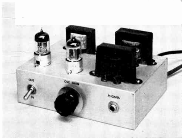
Fig. 8-10 — A combination c.w. monitor and code-practice oscillator that can be used without modification of the receiver or transmitter.
