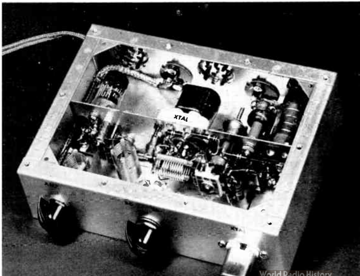
Fig. 19-8. The input tuning capacitor ( C_1 ), the antenna-heater switch ( S_1 ), and the low-frequency crystal ( V_2 ) are in line from left to right on the front wall of the chassis. A metal partition, mounted along the center line of the chassis, supports the tubes, the v.h.f. crystal ( V_1 ), and most of the r.f. components.
