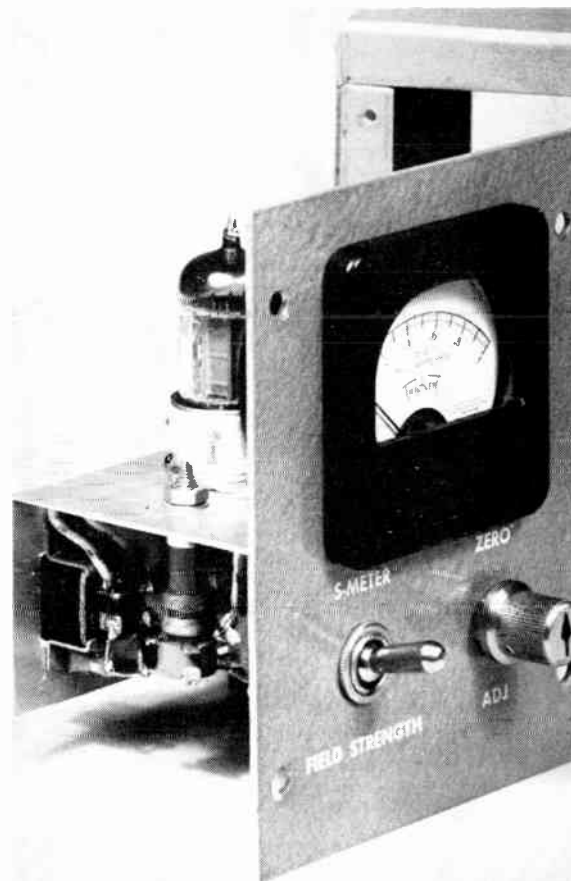
Fig. 19-51 — A front view of the signal/field-strength meter. The zero-adjust control is to the right of the toggle switch, S_1 . The meter registers either signal or field strength, depending upon the setting of the toggle switch.
