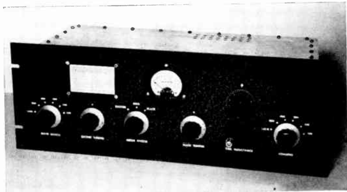
Fig. 6-48 — Controls, from left to right, are for band switch, exciter tuning, meter switch, pi-section tank capacitor, rotary inductor and turns counter, and output-capacitor switch. The panel is 7 by 19 inches. The top cover (a chassis bottom cover) is in place in this view.
