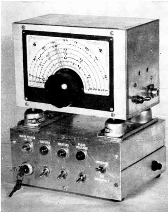
Fig. 6-62 —The v.f.o. remote tuning unit and control box. The tuning unit is enclosed in a 5 × 6 × 9-inch aluminum box mounted on shock absorbers. The control-unit enclosure is made up of two 7 × 9 × 2-inch aluminum chassis, bottom to bottom. The range-control switch and remote cable connector are mounted on one end of the tuning unit. A fuse holder projects from the end of the control unit.
