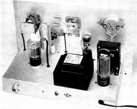
Fig. 6-37 — Rear view of the transmitter showing the placement of components above chassis. The loading capacitor, C_s , is at the left, L_3 is the vertical coil and L_2 the horizontal one. Rubber grommets are used to prevent chafing and to furnish additional insulation on the leads coming from below chassis.
