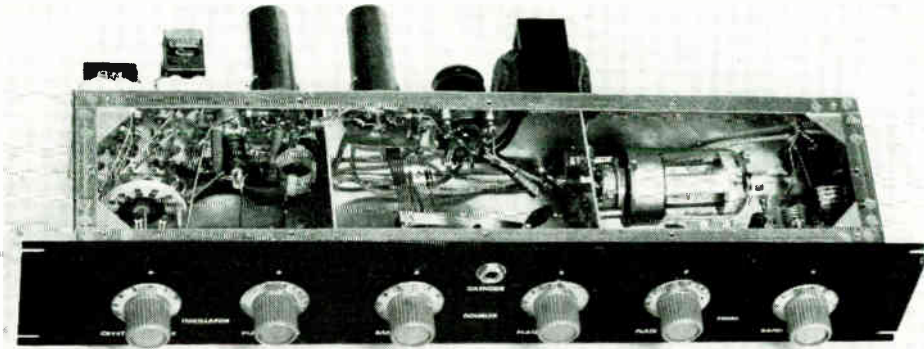
Fig. 17-2 — Looking into the handswitching exciter-transmitter from the top front. Oscillator components are in the left compartment, the doubler and power connector in the center, and the output stage at the right. Note that the 6146 socket is mounted inside the output stage compartment.
