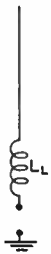
Fig. 20-33 — The capacitive reactance at frequencies lower than the resonant frequency of the whip can be canceled out by adding an equivalent inductive reactance in the form of a loading coil in series with the antenna.
