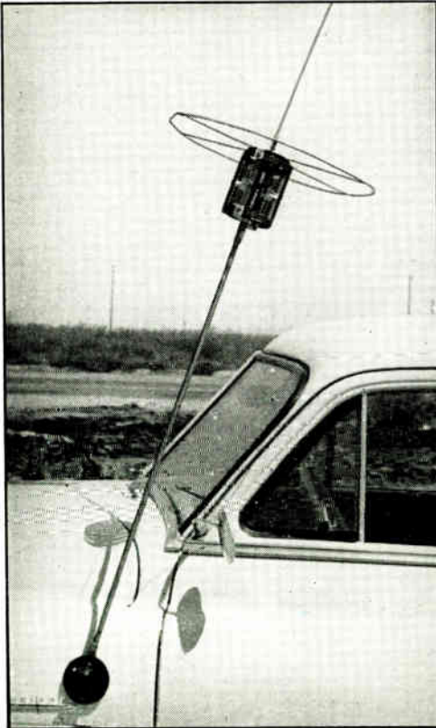
Fig. 20-37 — The top-loaded 4-Mc. antenna used by W6SCN. The loading coil is a B & W transmitting coil. The coil can be tuned by the variable link which is connected in series with the two halves of the coil.
