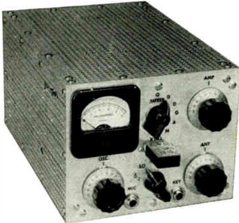
Fig. 20-16 — Front view of the 6-band mobile transmitter. The control knob for S_2 is located in between the meter and the dial for C_3 and C_4 . S_1 is directly below the crystal socket, with the knobs for C_2 and C_5 to the left and right, respectively. J_1 and J_5 are at the bottom of the 4\frac{1}{8} \times 6\frac{1}{4} -inch panel. The perforated aluminum cover is 9\frac{1}{8} inches deep and has a hole punched in the left side to permit adjustment of C_1 .
