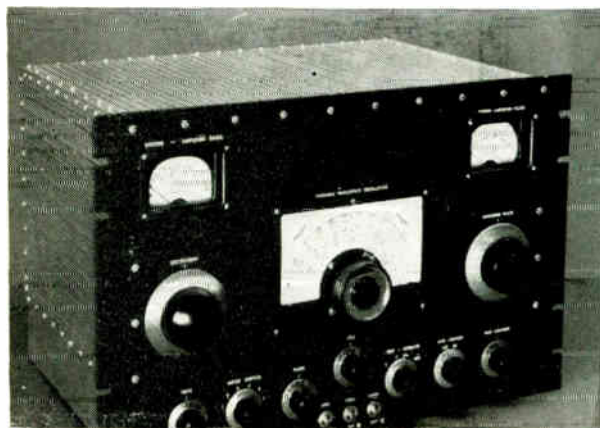
Fig. 6-61 — The standard-rack panel is 12\frac{1}{4} inches high. Controls (National HRS) along the bottom, centers spaced at intervals of 2\frac{1}{8} inches either side of center, are, left to right, for C_4 , S_2 , C_5 , C_2 , S_1 (Centralab 1405), S_2 and C_{10} . Power toggles are below at the center, spaced 1 inch apart. The calibrated VFO dial (National SCN) for C_1 is at the center, with the excitation control (National P dial) to the left, and the dial (National AM) for C_9 to the right. National CFA chart frames outline the rectangular openings for the recessed meters, 50-ma. to the left, 500-ma. to the right. The shielding enclosure is built up using aluminum angle, perforated sheet (also used for the bottom plate), and self-tapping screws.
