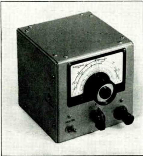
Fig. 20-9 — A bandswitching converter for 6, 10 and 11 meters. The pilot light at the lower right has an adjustable beam, for convenience in mobile work.
