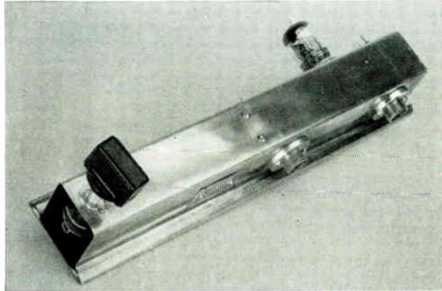
Fig. 16-24 — A highly effective r.f. amplifier for 420 Mc. The tank circuit is a half-wave line made of flashing copper. Coaxial fittings are for input and output connections. Heater and plate voltages are brought in on feed-through by-pass capacitors just visible on either side of the 6AJ4 tube.
