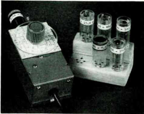
Fig. 21-20 — A compact and light-weight grid-dip meter for one-hand operation. It is built in a 1\frac{5}{8} \times 2\frac{1}{8} \times 4 -inch "Channel-lock" box and uses six plug-in coils to cover the range 1600 kc. to 160 Mc. The power supply and milliammeter for reading grid current are in a separate unit.
