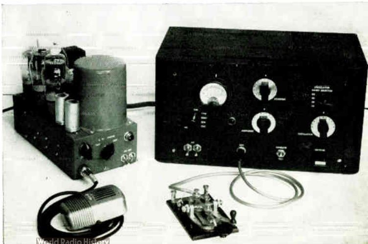
Fig. 9-16 — The 40-watt modulator alongside the 75-watt transmitter described in the transmitting chapter. It is completely self-contained, with power supply and control circuits, on a 5 × 10 × 3-inch chassis.
