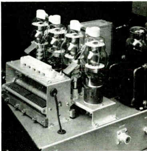
Fig. 12-19 — Close-up view of the plate circuit with the tank coil removed to show the blocking condensers, parallel-feed plate chokes and parasitic-suppressor coils. The double lead through the grommets runs from the output-circuit coil to the coupling condenser and coax connector underneath the chassis.
