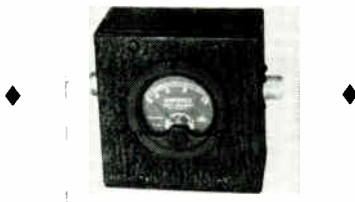
Fig. 21-28 — R.f. ammeter mounted for connecting into a coaxial line for measuring power. A "2-inch" instrument will fit into a 2 \times 4 \times 4 metal box. The shunt capacitance of an ammeter mounted in this way has a negligible effect on the accuracy at frequencies as high as 30 Mc. if the instrument has a bakelite case. Metal-cased meters should be mounted on a bakelite panel which can in turn be mounted in a cut-out which clears the meter case by about \frac{1}{4} inch.
