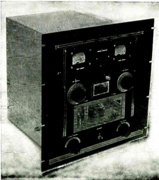
Fig. 6-89 - Front view showing the panel layout. Controls along the bottom are S_2 (coarse coupling), filament switch and grid-tuning. Above the window are the controls for C_{13} (fine coupling) and plate tuning. Between the meters is the counter dial on L_1 . The input and output connectors are along the left drop of the chassis. The hole in the center of the perforated top cover is for access to C_{10} . The chrome strips cover the 6-32 machine screws that fasten the angle to the panel. National CFA chart frames are used to cover the meter openings, and one is placed between the plate and output controls to use as a tuning chart. The bottom of RFC_2 shows between the tube bases, through the screened opening.
