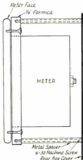
Fig. 6-65 — Sketch showing method of mounting meters in shielding boxes. The meters are suspended from the rear covers.
