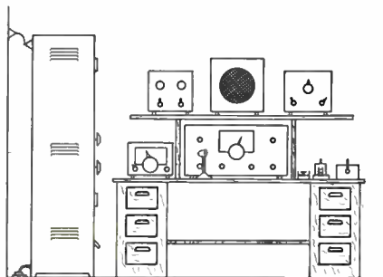
Fig. 22-1 — In a station assembled for maximum ease in frequency or band changing, the transmitter should be located next to the operating position, as shown above. On the operating table, the receiver is in front of the operator and VFO or crystal-switching oscillator on the left. (The VFO or crystal oscillator could be part of the transmitter proper, but most operators seem to prefer a separate VFO.)
