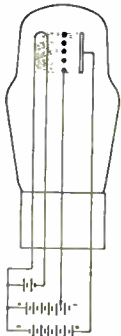
Fig. 3-5 — Construction of an elementary triode vacuum tube, showing the filament, grid (with an end view of the grid wires) and plate. The relative density of the space charge is indicated roughly by the dot density.
