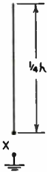
Fig. 20-31 — The quarter-wave whip at resonance will show a pure resistance at the feed point X.
