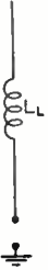
Fig. 20-36 — Placing the loading coil at the center of the whip antenna, instead of at the base, increases the radiation resistance, although a larger coil must be used.
