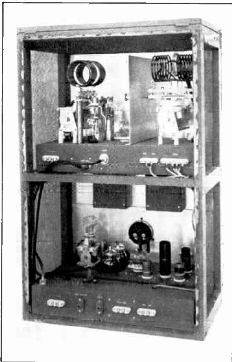
Fig. 6-59 — Rear view of the completed 500-watt all-band transmitter with the back screening panel removed. The rectangular enclosed unit to the rear of the exciter contains the v.h.f. power-lead filters. The two matching boxes above enclose the amplifier-stage milliammeters.
