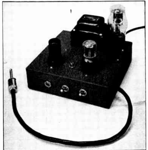
Fig. 8-11 — A top view of the "Monitone." The shaft of the screwdriver-adjusted potentiometer controlling tone and volume is located between the 6J5 and 6SL7 tubes. The right-hand switch controls the a.c., and the center switch cuts the tone oscillator in and out.
