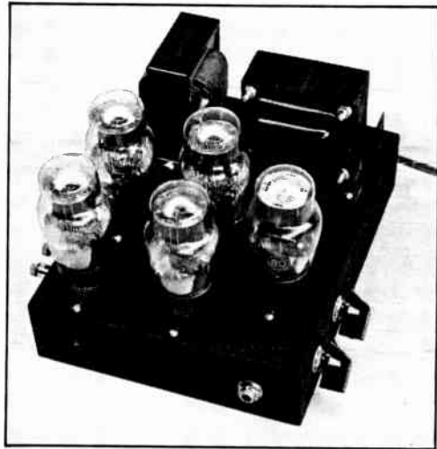
Fig. 8-9 — A vacuum-tube keyer, built up on a 7 X 9 X 2-inch chassis with space for four or less keyer tubes and the power-supply rectifier. The resistors and condensers that produce the lag are underneath, controlled by the knobs at the right. The jack is for the key, while terminals at the left are for the keyed circuit.
