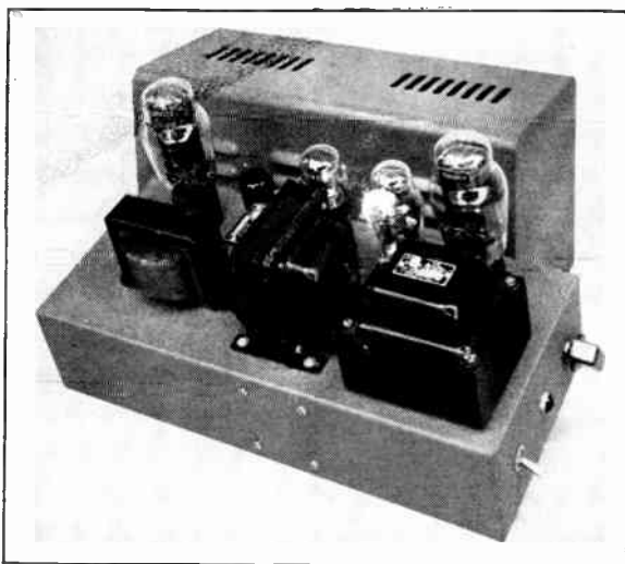
Fig. 7-17 — A heavy-duty electronically-regulated power supply. The unit is assembled on a 6 × 14 × 3-inch chassis fitted with an enclosing cover. The five tubes across the rear, left to right, are the 6AS7G regulator, the 6SJ7 control tube, the VR-105 bias regulator, the 1-V bias rectifier and the 5U4G power rectifier. In the foreground are the two filter chokes and the power transformer. The remainder of the components are mounted underneath.
