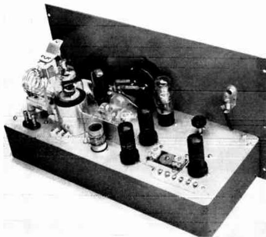
Fig. 6-54 — Rear view of the 75-watt all-band transmitter or exciter. The v.h.f. trap is fastened to the top of the tubular condenser, C_{39} , to the rear of the output tank coil and alongside the 807 and the 6V6GT. A small baffle shield separates the two multiplier coil sockets, shown here with the 28-Mc. bandpass coupler in place. The mounting of the low-frequency coupler is shown between the oscillator tube and the two frequency multipliers.
