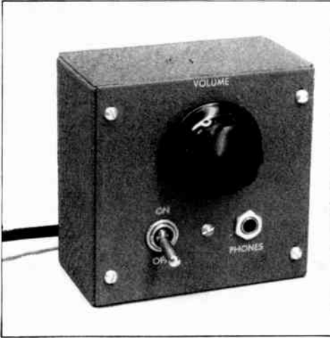
Fig. 5-39 — A simple audio noise limiter for reducing operator fatigue caused by ignition noises, key clicks and static crashes.
