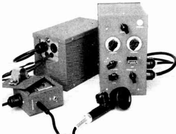
Fig. 6-116 — A compact 20-watt mobile transmitter for the 3.5- and 7-Mc. bands. Designed for mounting under the dashboard of the car, the transmitter and its power supply occupy standard 5 \times 6 \times 9 -inch utility boxes, and the control box, which clamps to the steering post, is in a 1 \times 1 \times 2 -inch box.
