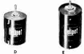
MODELS D AND E HELIPOTS Provide extreme accuracy of control and adjustment, with 9,000 and 14,400 degrees of shaft rotation. D —25 turns, 234" coil, 3-5 16" dia., 15 watts—resistances from 100 to 750,000 ohms. E —40 turns, 373" coil, 3-5 16" dia., 20 watts—resistances from 200 ohms to one megohm. — Ask for Bulletin 104 —
