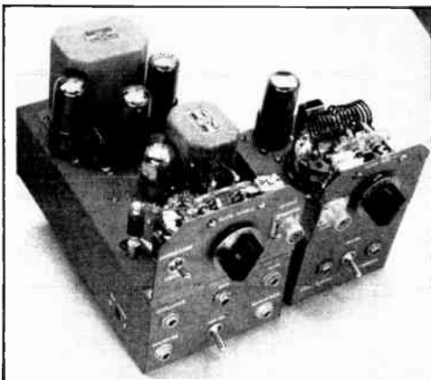
Fig. 13-37—A 2-band set-up for mobile or low-powered fixed-station operation on 50 and 144 Mc. At the left is the 2-meter unit, complete with modulator. The smaller is the 50-Mc. r.f. section. Toggle switches permit use of the modulator with either r.f. section.
