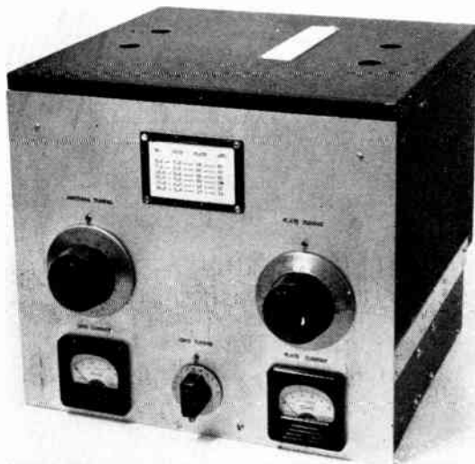
Fig. 6-94 — A multiband push-pull 807 amplifier and antenna tuner with no plug-in coils or switching. The aluminum strip on top covers the harmonic-trap adjusting holes. The other holes are for ventilation. The panel is a sheet of \frac{3}{16} -inch aluminum 12\frac{1}{4} inches wide and 10\frac{1}{2} inches high.
