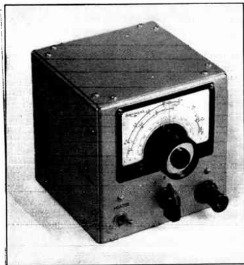
Fig. 12-22 — A bandswitching converter for 6, 10 and 11 meters. The pilot light at the lower right has an adjustable beam, for convenience in mobile work.
