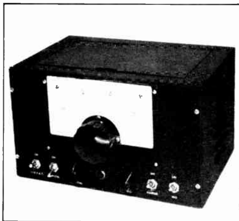
Fig. 16-3 — Additive frequency meter with self-contained power supply. The small knobs are for correction of drift so that both the 100-ke. crystal oscillator and VFO can be set to exact frequency. Dial calibration is in 1000-cycle intervals. This unit can be used for high-accuracy frequency measurement at all frequencies from 100 ke. through 30 Mc.
