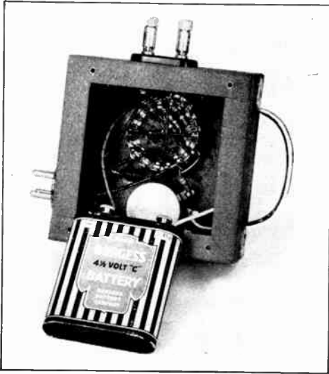
Fig. 16-19 — A rear view of the volt-ohm-milliammeter. The range-selector switch is mounted above the zero-adjustment potentiometer, and the shunts and multipliers are connected across the switch terminals. A four-prong male plug, for connection to the meter box, is shown at the left of the cabinet. The ohmmeter battery fits inside the case; the battery terminals should be insulated with tape or paper before the battery is installed in the box.
