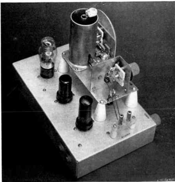
◆ Fig. 12-19 — Rear view of the superregenerative receiver. The r.f. circuits are mounted on a copper shelf to the left of the antenna terminals. The detector tuning condenser is mounted on a small panel to the front of the coaxial line, and the band-set condenser is soldered across the open end of the line. The r.f. stage is mounted on an "L"-shaped bracket with the tube socket and plate-circuit components on the left side and the grid circuit on the right side. Audio tubes and voltage regulator are in line across the rear of the chassis.
