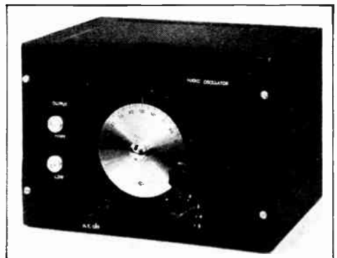
Fig. 16-30 — Variable-frequency audio signal generator. A dial of the type permitting direct calibration can be substituted if desired. This instrument is complete with power supply and covers the 30–15,000 cycle range in five steps.
