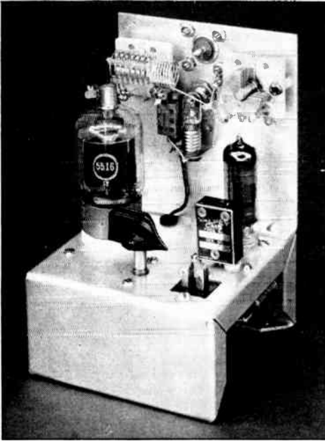
Fig. 13-29 — Rear view of the 50-Mc. r.f. section. The knob above the chassis is the cathode control. The final tank circuit is at the upper left, with antenna series tuning at the upper right.
