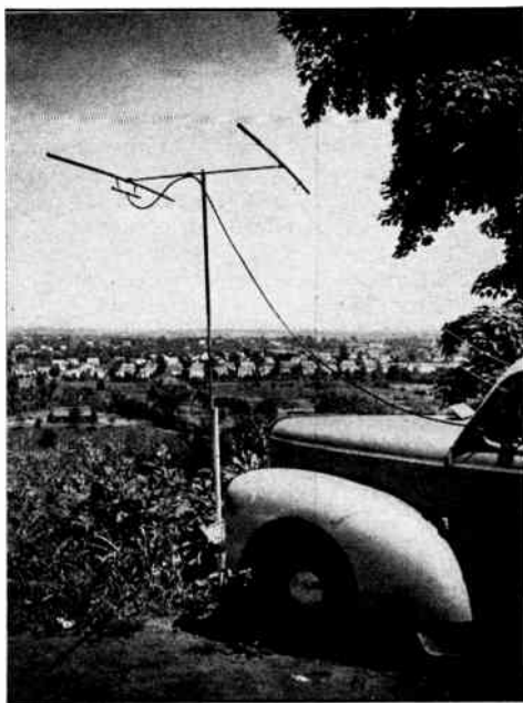
Fig. 14-12 — A 2-element collapsible array for 50-Mc. portable use.
