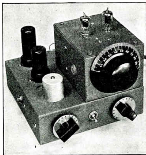
Fig. 1417 — Left — The 112-Mc. t.r.f. superregenerative receiver uses a 9001 in the r.f. stage, 9002 detector, 6J5 first audio, and 6F6 output stage. The knobs along the front are audio volume control (left) and the regeneration control. The rubber grommet on the side of the 3 \times 4 \times 5 -inch box centers the screwdriver used for setting the detector hand-set condenser; a similar one is provided on the other side for the r.f. hand-set adjustment. Note the 'phone jack on the side; the speaker terminals are located at the rear. Right — A view under the chassis of the t.r.f. receiver shows the audio transformer and the arrangement of some of the other components. The three wires coming through the chassis to the right of the "B" + switch are the leads from the r.f. section of the receiver.
