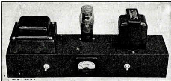
Fig. 1505 — The power-supply chassis also houses the milliammeter for all plate-current measurements in the 56-Mc. transmitter.
