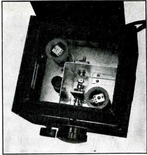
Fig. 1127 — Top view of the preselector. The padder condensers are mounted inside the plug-in coil forms.
