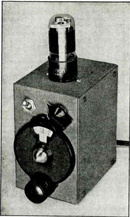
Fig. 1908 — A 50-, 100- and 1000-kc. electron-coupled frequency standard, using a dual-purpose 117L7GT tube which serves as both rectifier and oscillator. It is built up complete with transformerless power supply in a 3 x 4 x 5-inch metal box. The controls are the main tuning dial, power on-off switch, and frequency selector switch.
