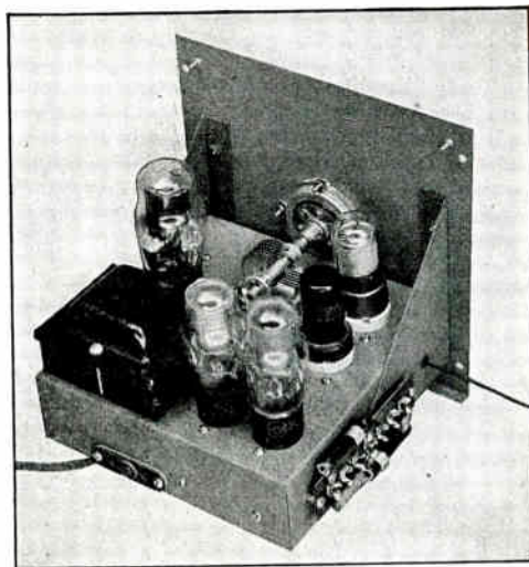
Fig. 1907 — Rear view of the electron-coupled heterodyne frequency meter. The 7 X 7 X 2-inch chassis is supported by two brackets for rigidity. It is raised sufficiently to accommodate the height of the coil shield underneath; this also enables mounting the tuning condenser directly on the chassis. The voltage-divider resistors are mounted outside to keep heat from the coil.
