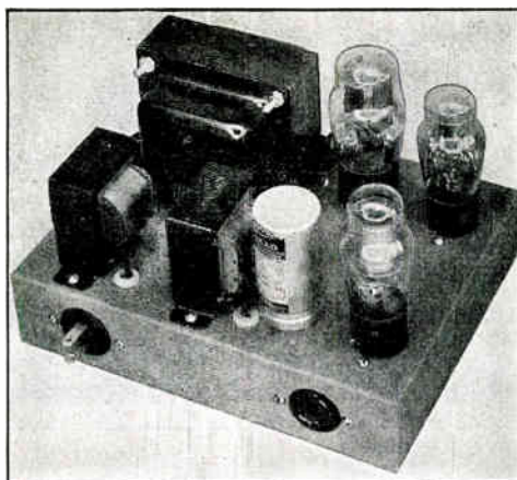
Fig. 1236 — A combination power-supply unit delivering 250 or 300 volts for exciter plate-supply and 75 volts of fixed bias. The unit is designed especially to work with the band-switching exciter of Fig. 1232 or the transmitter of Fig. 1221. If desired, the components may be combined with the components for a high-voltage plate-supply on a single chassis. The circuit diagram of the combination unit is shown in Fig. 1237.
