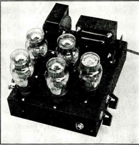
Fig. 1290 — A vacuum-tube keyer, built up on a 7 \times 9 \times 2 -inch chassis with space for four or more keyer tubes and the power-supply rectifier. The resistors and condensers which produce the lag are mounted underneath, controlled by the knobs at the right. The jack is for the key, while terminals at left are for the keyed circuit.
