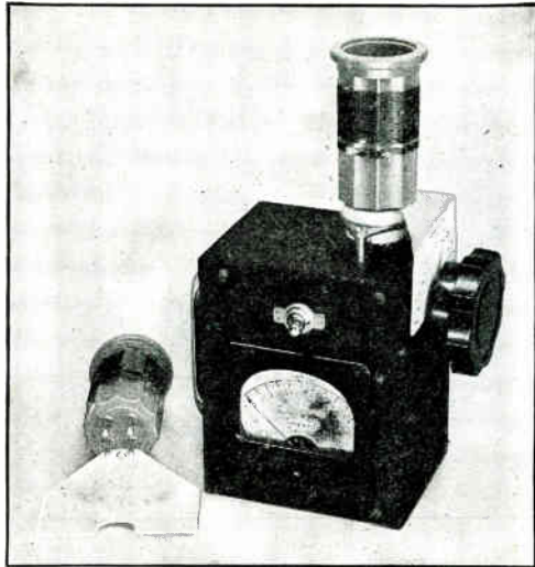
Fig. 1903 — A sensitive absorption-type frequency meter with a crystal-detector rectifier and d.c. milliammeter indicating circuit. Individual calibration charts mounted directly on each coil form make the meter direct-reading. The toggle switch places a 10-ma. shunt across the 0-1 ma. meter; this range is used for preliminary readings, to avoid burning out meter or crystal. The meter gives indications at several feet from a low-power oscillator.
