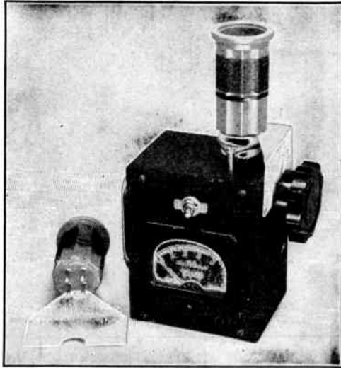
Fig. 1804 — A sensitive absorption frequency meter with a crystal-detector rectifier and d.c. milliammeter indicating circuit. Individual calibration charts mounted directly on each coil form make the meter direct-reading. The toggle switch places a 10-ma. shunt across the 0-1 ma. meter; this range is used for preliminary readings, to avoid burning out meter or crystal. The meter gives indications several feet from a low-power oscillator.
