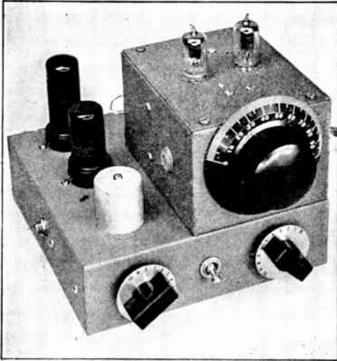
Fig. 1418 — Left — The 112-Mc. t.r.f. superregenerative receiver uses a 9001 r.f. stage, 9002 detector, 6J5 first audio and 6F6 output stage. The knobs along the front are audio volume control (left) and regeneration control. The rubber grommet on the side of the 3×4×5-inch box centers the screwdriver used for setting the detector band-set condenser; a similar one is provided on the other side for the r.f. band-set adjustment. Note the 'phone jack on the side; the speaker terminals are located at the rear. Right — A view under the chassis of the t.r.f. receiver shows the audio transformer and some of the other components. The three wires coming through the chassis to the right of the "B"-plus switch are the leads from the r.f. section of the receiver.
