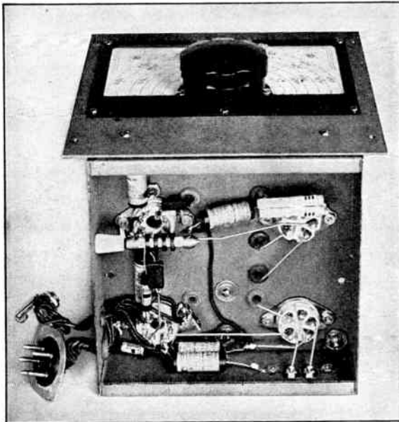
Fig. 1255—High-frequency connections underneath the chassis of the v.f. exciter unit are made with short, straight sections of heavy wire. The two zero-temp padding condensers are soldered directly to the oscillator-coil socket. All components should be mounted firmly with no opportunity to support mechanical vibrations. Washers about \frac{1}{8} -inch thick should be placed between the panel and the chassis to provide space for the lower lip of the cabinet opening.
