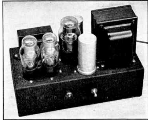
Fig. 1257 — Voltage-regulated power supply for the v.f. exciter unit. One filter choke is mounted underneath the chassis.
