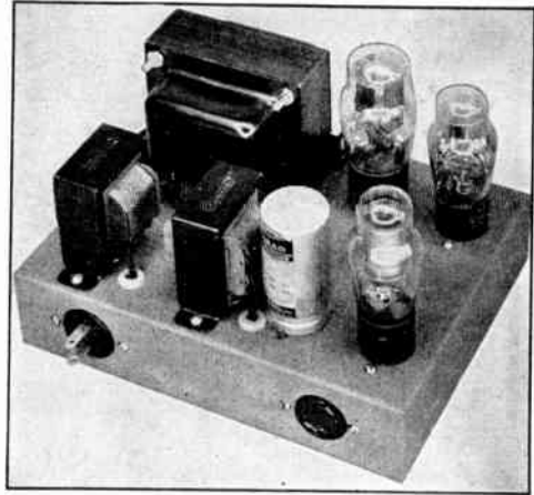
Fig. 1236 — A combination power-supply unit delivering 250 or 300 volts for exciter plate supply and 75 volts fixed bias. The unit is designed especially to work with the bandswitching exciter of Fig. 1232 and the transmitter of Fig. 1221. If desired, the components may be combined with high-voltage plate-supply components on a single chassis. The circuit diagram is shown in Fig. 1237.
