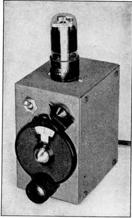
Fig. 1808 — A 50-, 100- and 1000-kc. electron-coupled frequency standard, using a dual-purpose 117L7GT tube that serves both as rectifier and oscillator, complete with transformerless power supply in a 3 × 4 × 5-in. metal box. The controls are: main tuning dial, power switch and frequency selector switch.
