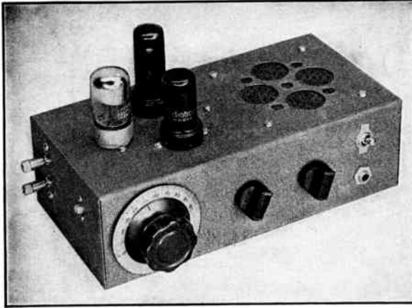
Fig. 1622 — A superregenerative receiver with built-in speaker. The detector trimming condenser is mounted on the side. The audio gain control is mounted next to the tuning control (extreme left) and the regeneration control is between the volume control and the 'phone jack and on-off switch.
