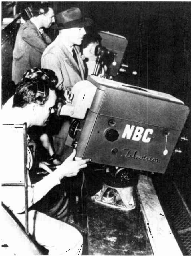
RCA's new image-orthicon cameras allowed better coverage of sporting events. ( National Archives )
