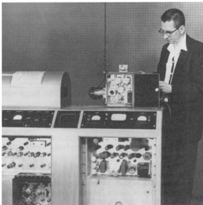
John Boor, director of engineering at KCTS-TV Seattle, works on a 1955-vintage kinescope recorder.
