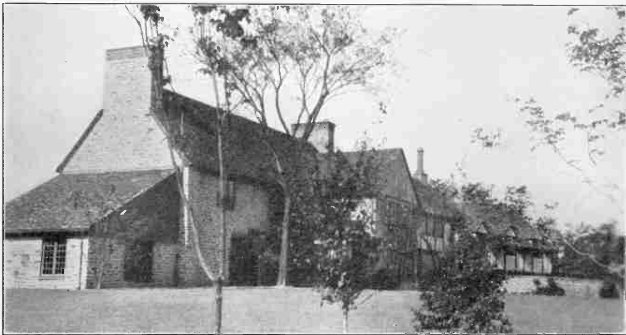
FIG. 2.—The same scene reproduced with 100 screen, or 10,000 elements per square inch. Despite the substantial reduction in the number of elements, the sacrifice of detail is moderate.
