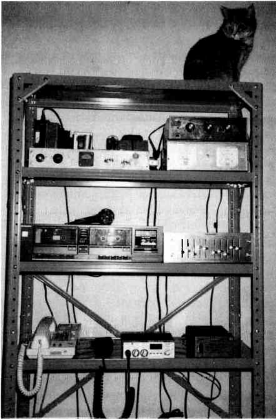
Fig. 4-3. WCPR uses this homemade 35-watt transmitter and other audio equipment (the unnamed housecat apparently does not hold a position within the station).
