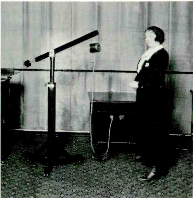
This 1921 picture shows an early microphone with a boom arrangement that permitted it to be raised or lowered according to the performer's height.
