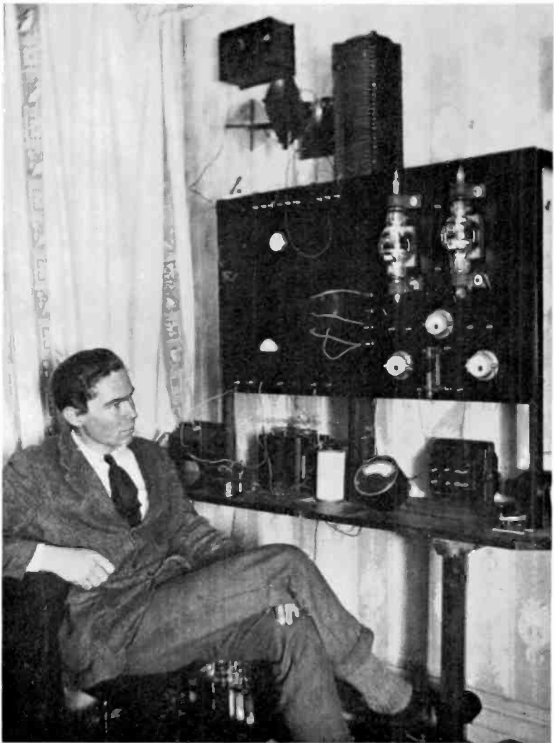
Hugh Ryan, 5BV, with the 100 metre transmitter he used during December 1923 when signals from his station were among the first to be heard in the United States. In terms of contact, as distinct from two-way working, he was probably first across from the United Kingdom as he exchanged call signs with American 8AJW on December 2, 1923, on 200 metres.
