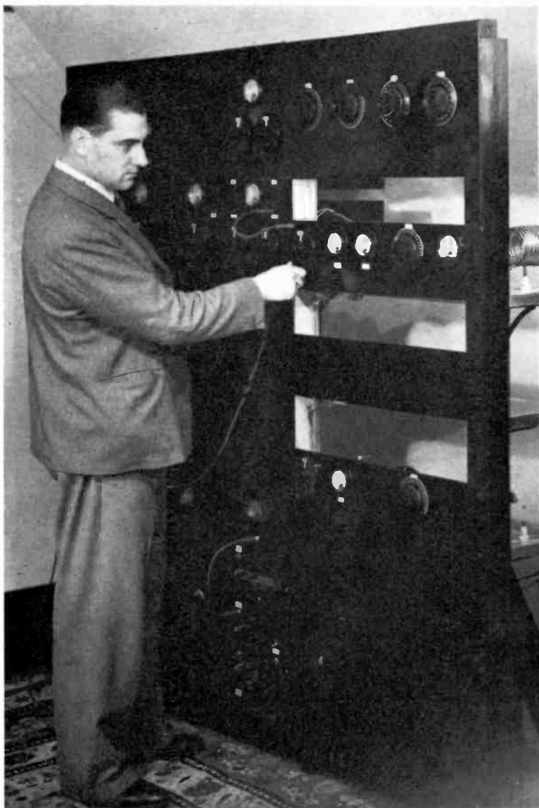
The transmitting equipment used by J. W. Mathews, G6LL, during the period 1937-1939 was housed in a wooden frame with plywood panels and metal chassis. The 14 Mc/s power amplifier used a pair of RK 20 valves, suppressor modulated. The panel on top with four dials carried the aerial tuning unit circuits for four bands, each pre-set for rapid band changing. The stages were all link-coupled by means of standard plugs and jacks—there were no coaxial plugs, or coaxial cable, at that time.
