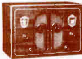
MODEL 355 —Left for A. C.—D. C. Current and 1 MODEL 350 (Right for A. C. Current—5 tube, 8 tube performance) Dual Wave Vibro-Power superheterodyne Personal Radio. Portable. Size 11 1/2" wide x 7 1/2" high x 8 1/2" deep. Built-in antenna. Range 530 to 3,200 Kilocycles (408 communication channels). Full automatic volume control. Illuminated eye-level control. 3-gang condenser. 8 to 1 reduction for tone control. Illuminated 2-color calibrated dial. Full floating coil large size dynamic speaker. For Underwriters' Laboratories Approval. R.M.A. steel. Solid heavy metal. Mahogany cabinet with genuine inlay. Hand-rubbed piano finish and full wood look. $37.50
