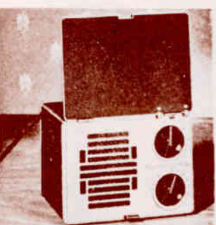
MOTOROLA 3A5 PERSONAL PORTABLE radio, "P" design, operates on ac-dc or battery. Weighs 6 lbs. Employs 5 tubes (including rectifier). Tuning range covers 550 to 1600 kc. Line cord can be tucked away inside case when not in use. Set turns on when front cover is opened. Maroon finished metal with chrome trim measures 6 1/2 long, 4 1/2 high, 5 1/2 inches deep. Also available in Model A-1, battery operated only, list price $19.95. Galvin Mfg. Co., 4545 Augusta Blvd., Chicago, Ill.
