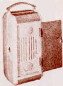
DETROLA PERSONAL PORTABLE 3-way radio operates on a.c. or battery. This 5-tube including one ballast tube, superhet is housed in tan marble finish, trimmed in grained Detrola to match. Measures 4 1/2 wide, 8 1/2 high, and 4 inches deep. Weighs approximately 4 lbs. Illustrated model 378, $19.95 complete.
