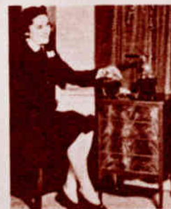
ANSLEY OXFORD DYNAPHONE is an 8-tube combination radio and automatic phonograph tuning short-wave and standard broadcast bands. Plays ten 12-inch or twelve 10-inch records. Mahogany cabinet with front panel of feathered crotch veneers and legs of solid mahogany. Measures 28 x 17 1/2 x 16 1/2 inches. The instrument panel is located in the top-lower-simulated drawer; the top opens to give access to the record changer. List price $129.50, ac operation. Ansley Radio Corp., 4377 Bronx Blvd., New York, N. Y.
