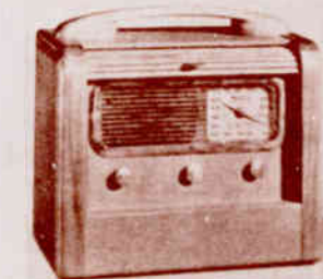
PHILCO 3-WAY PORTABLE radio, model 854-T, provides for short wave reception in addition to the standard American broadcast band. Cabinet finished with solid walnut has roll-top beaver-graining panel that can be opened or closed. Features non-inducing converter tube and two i-F stages. Tube circuit new simulated cork dial with foreign stations to be named by countries or cities. Philco Radio & Tele. Corp., Philadelphia, Pa.
