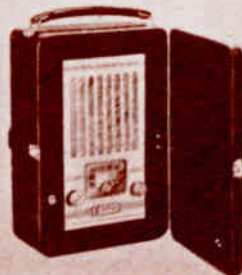
FADA PERSONAL PORTABLE radio, model C34, is a 3-way receiver operating on a.c. or battery. Has 5 tubes and covers American broadcast. Contains 4-inch speaker. Measures 9 high, 8 wide and 4 inches deep. Weighs 6 lbs. Housed in a black leatherette case. Set complete with batteries, $19.95. Fada Radio & Electric Co., Inc., 32-20 Thomson Ave., Long Island City, N. Y.
