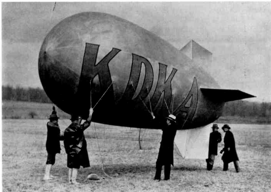
KDKA experiments with baloon antenna.
