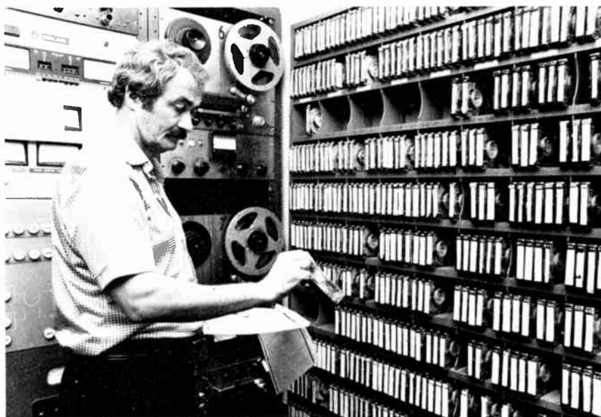
9.4. A KSFO engineer checks the various cartridges needed for the day's programming. Most stations keep hundreds of carts on hand for various commercials and promotional announcements, station IDs, and music. Photo by Nadine Ohara. Courtesy, KSFO radio, San Francisco.
