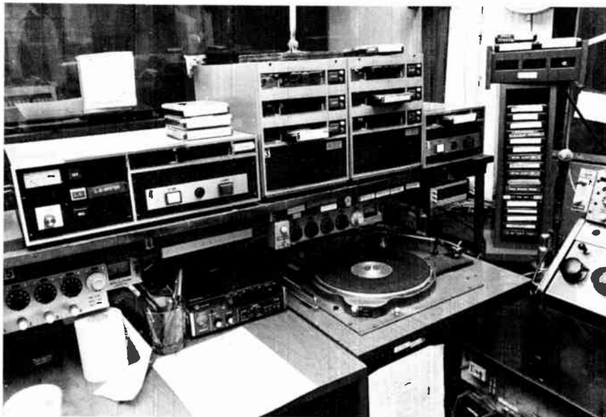
9.3. Another production room setup. The turntable is flanked on the left by a studio cassette machine and on the right by a cart rack. Above it is a battery of various cart machines. Photo by Nadine Ohara. Courtesy, KSFO radio, San Francisco.
