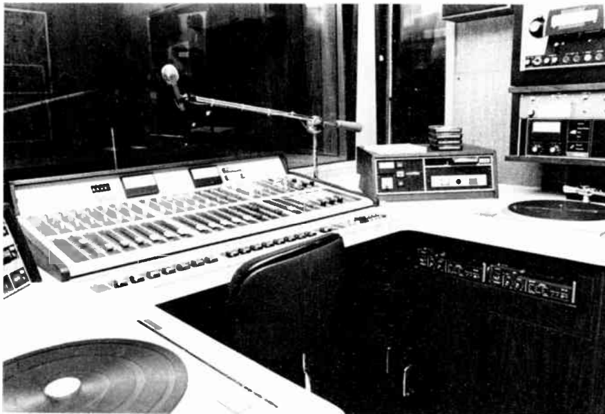
9.2. A standard production studio. The turntables are at the far left and far right. The mixing board is on the left, with the microphone just above it. Just to the right is the cart machine. Above the far right turntable is the bottom half of a studio reel-to-reel tape recorder and a VU meter. Photo by Nadine Ohara. Courtesy, KSFO radio, San Francisco.
