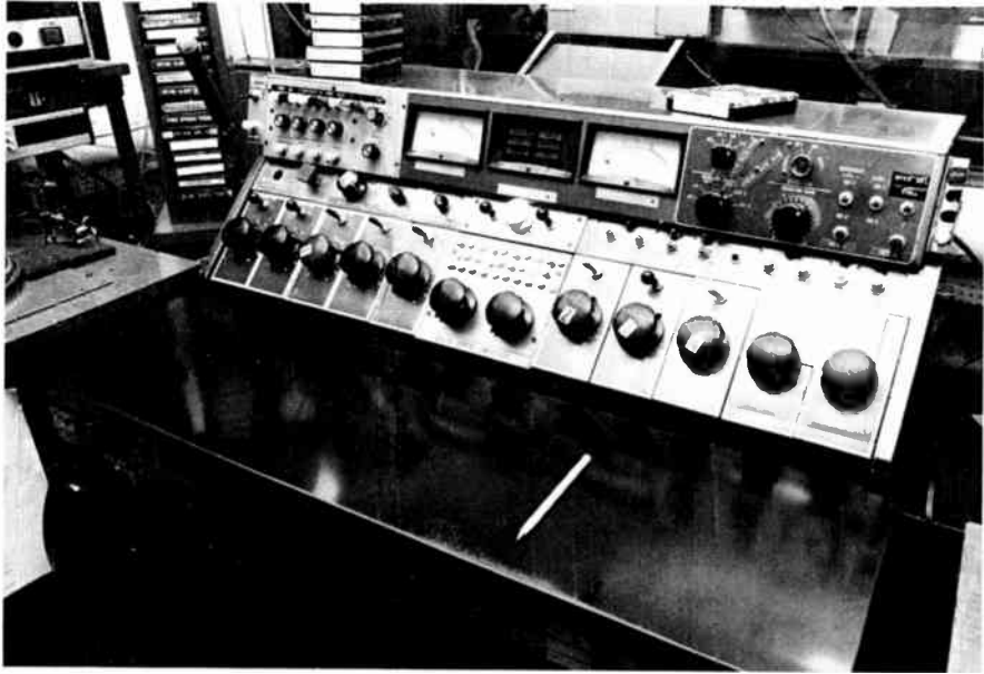
9.5. Sure, it looks like something out of Star Wars now, but with some practice, the mixing board can become a good friend. Note the numbered "pots," each of which is responsible for an input source. Photo by Nadine Ohara. Courtesy, KSFO radio, San Francisco.
