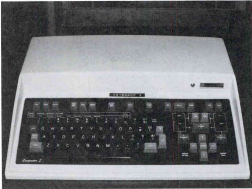
Picture 7-2. This is a keyboard for an electronic character generator. The layout of the keys is similar to a typewriter with the addition of several function and operating controls.
