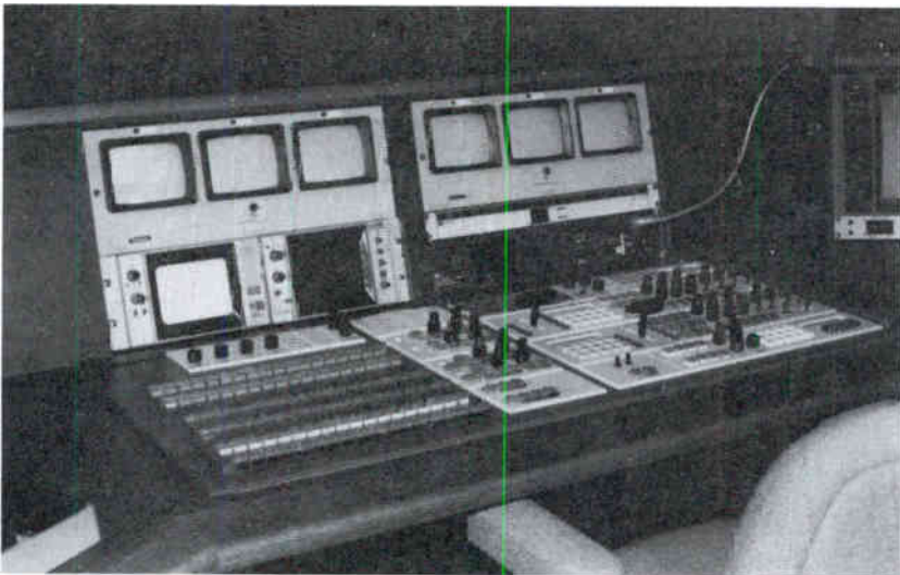
Picture 1-15. The central part of production control is the production switcher. The director operates the production switcher to select among the cameras during a program. The director should also have easy access to special effects, film and videotape recorder remote controls.
