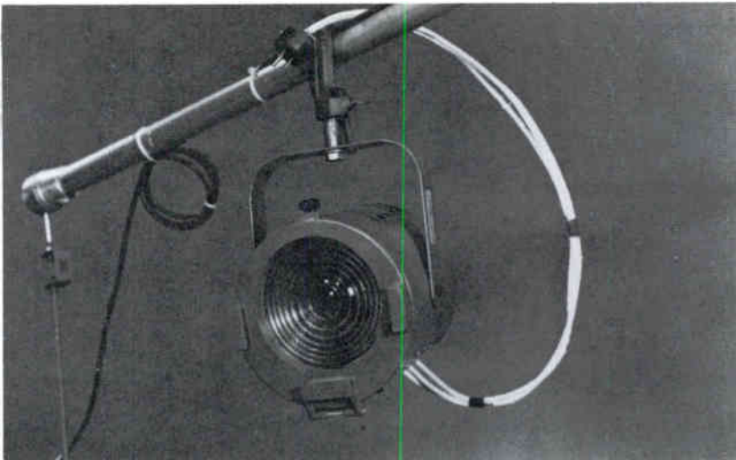
Picture 4-3. Fresnel spot lights are characterized by a high light output.
