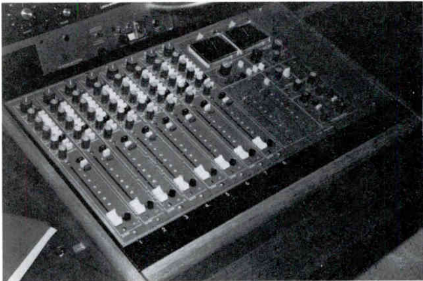
Picture 1-13. The heart of the audio system is the audio mixer. It brings all of the audio sources such as phonograph, audio tape, cartridge tape, and microphones together for mixing. The audio mixer has a knob or volume control for each source to permit proper mixing of each input.
