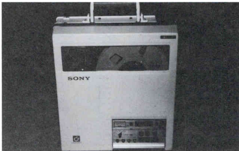
Picture 1-9. A remote videotape recorder is usually compact and capable of battery operation.
