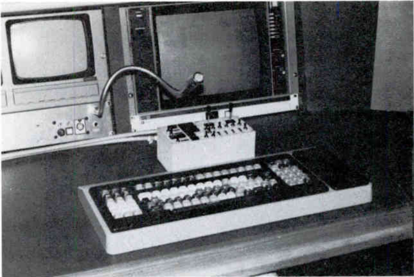
Picture 1-12. Sophisticated editing systems use computers to manipulate not only the VTR's, but also the production switcher.
