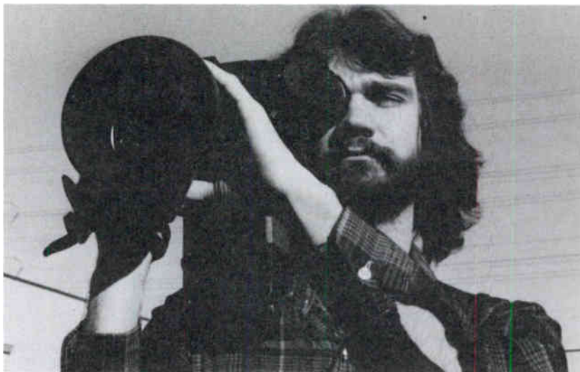
Picture 1-2. A portable camera is one which normally operates on batteries. It is often capable of “shoulder mounting” on the operator.
