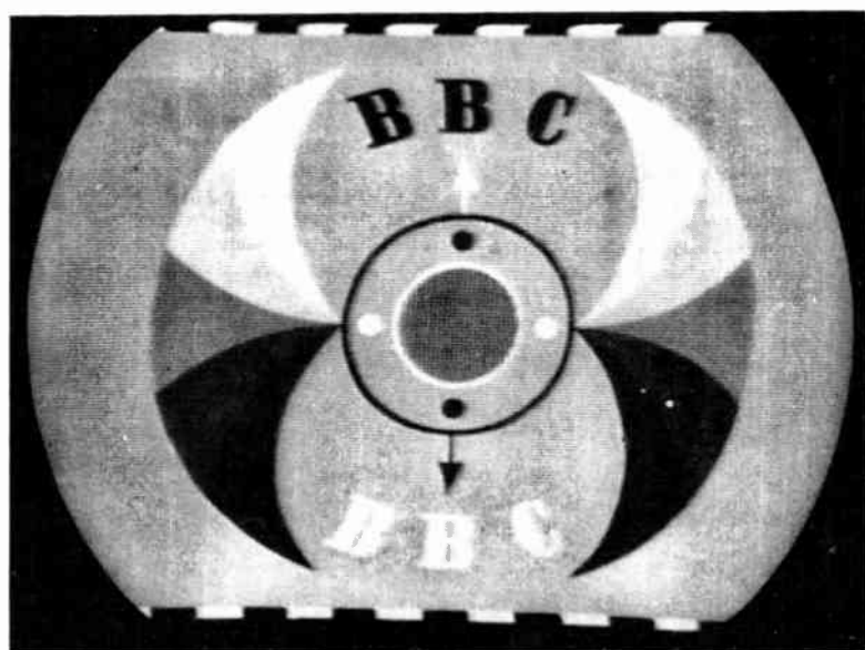
A reasonable reproduction of the tuning signal as received on an average receiver when the controls are adjusted properly
