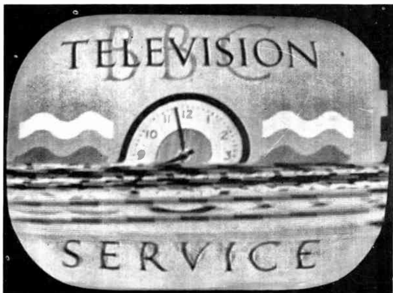
Effect of partial line slip. Adjust line (or horizontal) hold control
