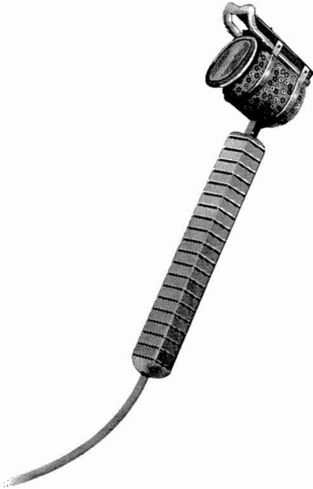
Fig. 17.1. The lip mic. The microphone has excellent noise-cancellation properties which makes it ideal for commentary situations. The mouthguard is held against the broadcaster's lip while the microphone is in use. There is a bass cut in the handle to compensate for the bass lift which results from working close to a ribbon microphone.
