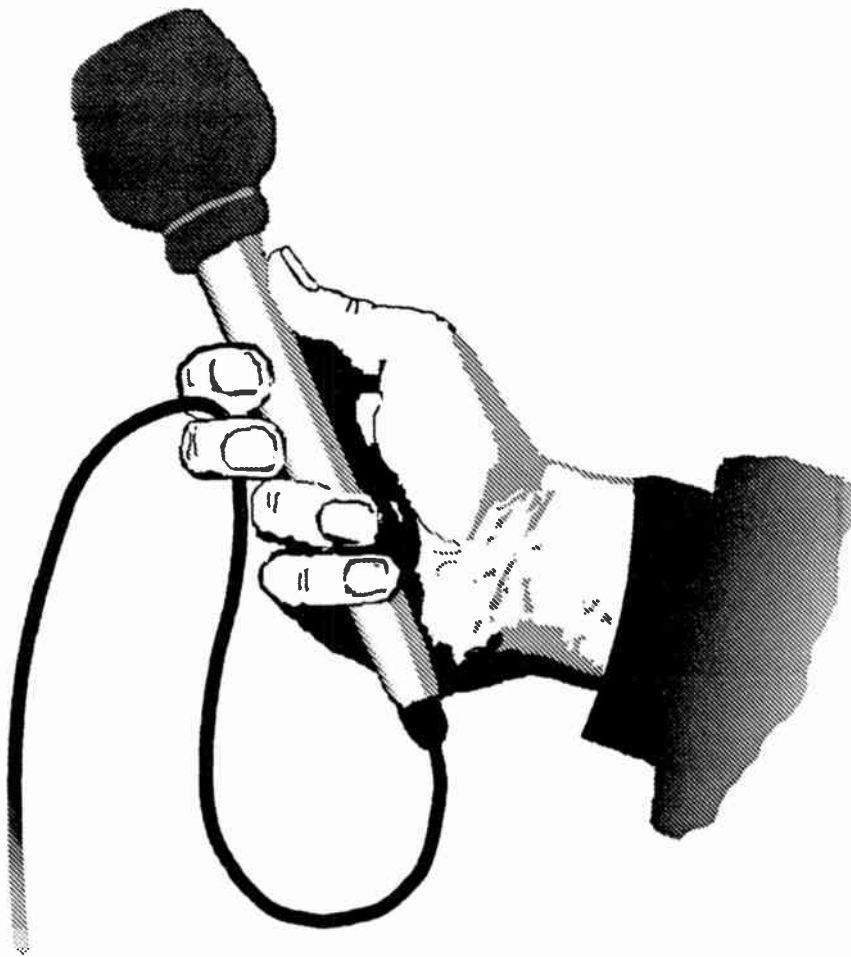
Fig. 3.3. The microphone cable is formed into two loops. The loop round the finger is kept away from the microphone case to prevent extraneous noises, commonly known as mic rattles, being passed along the cable. The windshield helps to prevent wind noise and voice 'pops'.
