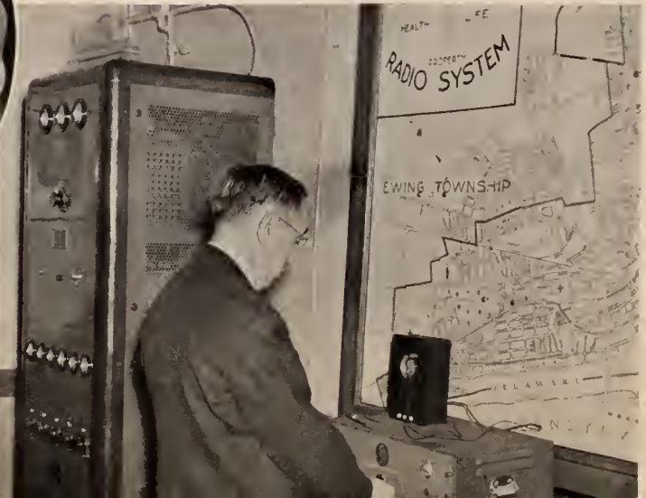
A monitoring unit is being used by this RCA engineer to check a police radio transmitter.
