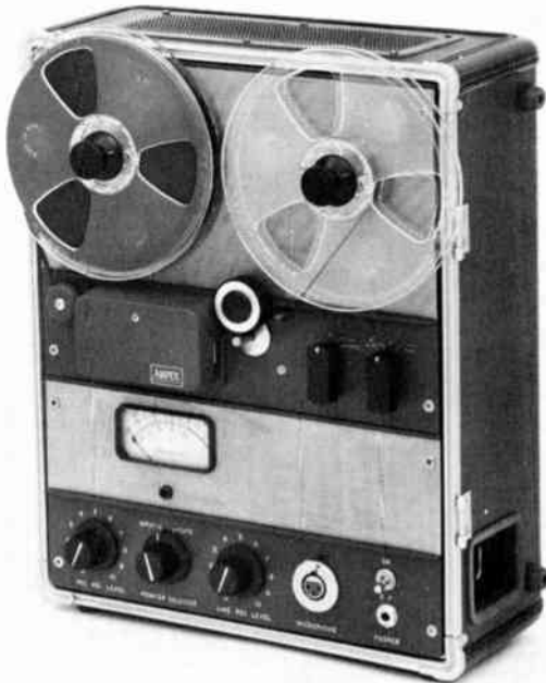
Fig. 6: Portable AC-operated broadcast-type tape recorder. Ampex 602.
