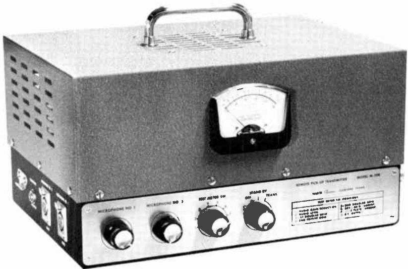
Fig. 9: Remote pickup radio transmitter for portable or mobile use. 150 megacycle band, FM, 30 watts output. Marti M-30B.
