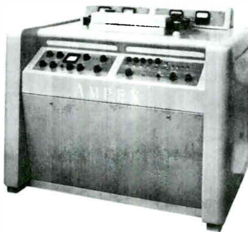
Figure 5.12 Ampex VR 1000. Ampex introduced this machine, the first commercially available videotape recorder, in 1956. Its 2-inch-wide tape was the standard for broadcast stations for years. (Photograph courtesy of Ampex Corporation. Used by permission.)
