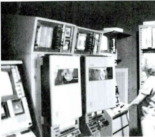
Figure 12.9 Open-reel and cartridge videotape recorders. Broadcast stations often playback (a) programs on open-reel (reel-to-reel) VTRs and (b) short segments (such as commercials and news stories) on cartridge machines. This video cartridge machine uses two stacks for loading the cartridges (you see one of them at left, partially obscured by the operator) and can be programmed in advance (keyboard and screen at right) for near-instant random access. In (a) the reels can be seen through the front glass of the VTRs' cases. In (b), a cartridge sits on the counter between the operator and the keyboard.
