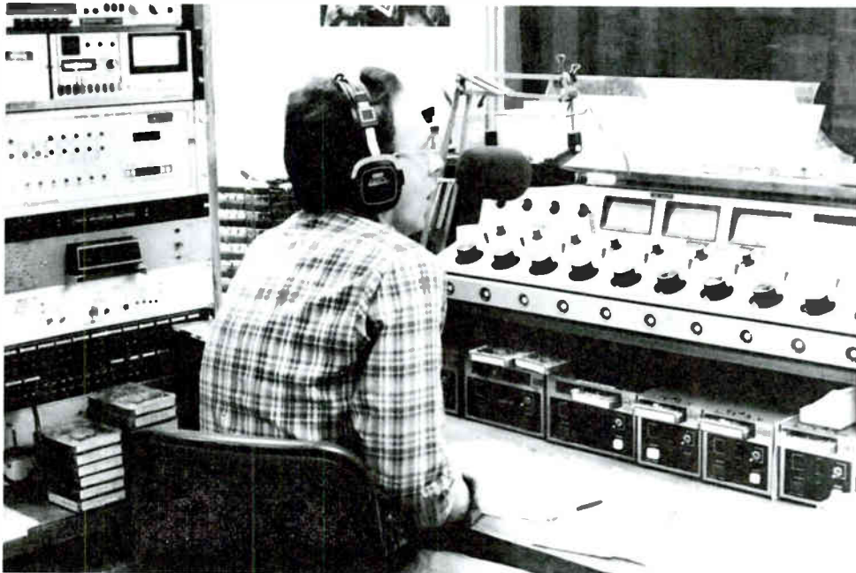
Figure 6.1 Radio combo operation. In front of the operator is the audio console. Meters at the top of the console indicate relative loudness of the audio signal. The microphone, over the console, is on an adjustable boom. Note the stack of audiotape cartridges (lower left) and the line of cartridge playback units (below the console); this station “carts” (transfers to audiotape cartridges) all records, and the operator plays the cartridges instead of records over the air.
