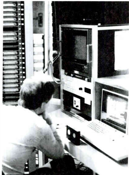
Figure 12.9 Open-reel and cartridge videotape recorders. Broadcast stations often playback (a) programs on open-reel (reel-to-reel) VTRs and (b) short segments (such as commercials and news stories) on cartridge machines. This video cartridge machine uses two stacks for loading the cartridges (you see one of them at left, partially obscured by the operator) and can be programmed in advance (keyboard and screen at right) for near-instant random access. In (a) the reels can be seen through the front glass of the VTRs' cases. In (b), a cartridge sits on the counter between the operator and the keyboard.
