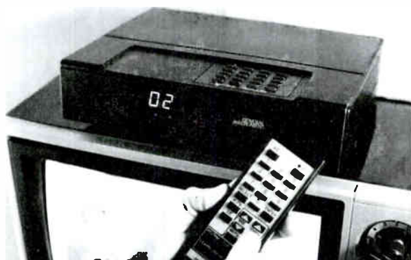
Figure 12.24 Cable adapter box. The subscriber end of the Jerrord IMPULSE 7000 system by General Instrument consists of this sophisticated, feature-packed addressable converter. The subscriber may operate the converter using either the control buttons on top of the box or the remote control. Among the many features of the IMPULSE 7000: channel selection; volume control; mute button; favorite-channel programming; last-channel recall; parental-control channel lock-out; time-controlled programming (for unattended VCR recording); response capability for video opinion polling; and both planned and impulse pay-per-view event buying. (Converter courtesy of Cox Cable-University City.)
