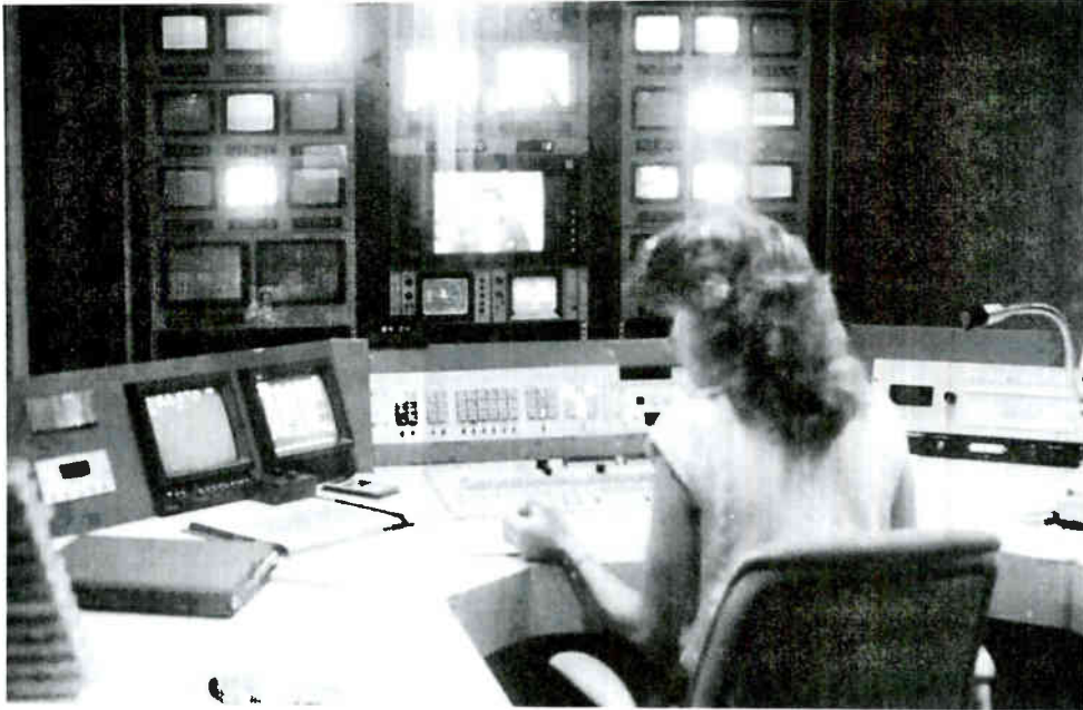
Figure 6.13 Duty director. At Orlando's Channel 2, the duty director's station is a centrally located, glass-enclosed booth. A computer feeds an electronic version of the program log to a video monitor (lower left). The switching equipment (lower center, in front of the duty director) handles video and audio simultaneously, so one person operates both. In the background—actually on the other side of the booth's glass wall—video monitors show the various program sources available.
