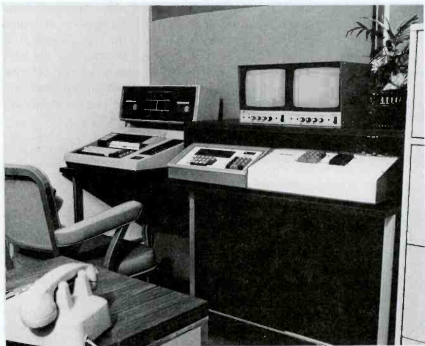
Figure 4.10 Traffic control center for WBEN-FM, Buffalo, New York, using Systems Marketing Corporation's DP-2 system. This system, using a micro-processor computer and a digitally controlled audio switcher and processor, can program the station for a full week. The twin monitors show current running program display but permit display of any part of the week's programming and allow for changes or additions to the memory instructions. Common with such systems are automatic logging, automatic network recording and playback, interfacing to other computers, and a master clock system.
