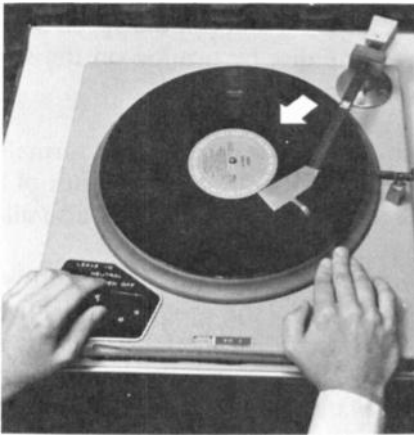
Figure 3.11. . . . then backtrack the plate a quarter-turn. Note that the speed selector has been put into gear.
