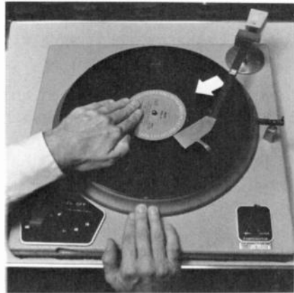
Figure 3.15. . . . and the record backtracked. The turntable is in gear and all set to go.
