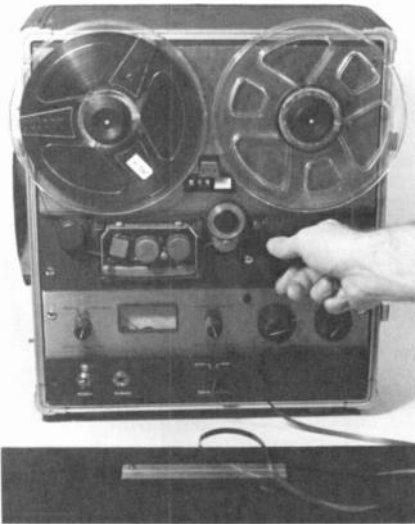
Figure 6.8. Spilling off tape after making the cut. You can do it this way . . .
