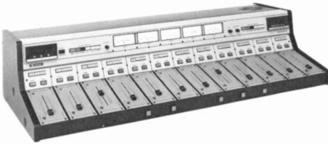
Figure 2.12. A broadcast audio console that uses slide faders. (Photo courtesy of Harris Corporation, Quincy, Ill.)
