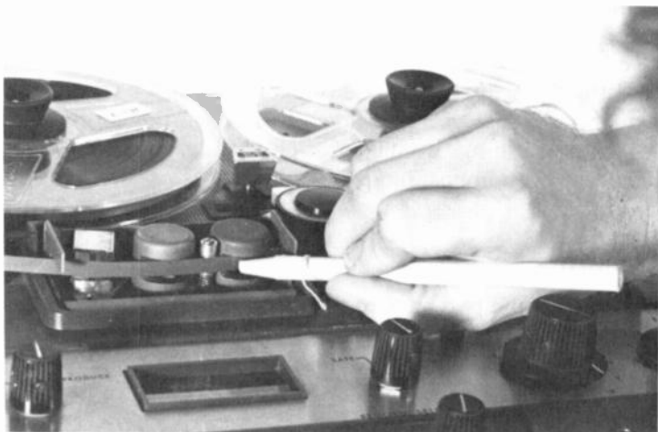
Figure 6.2. Marking the edit point. Be careful not to get grease pencil on the head.
