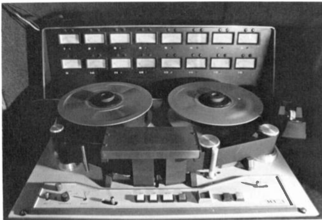
Figure 14.2. A tape machine using 2-inch audio tape, for multitrack recording.
