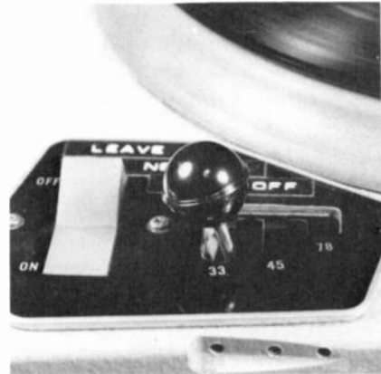
Figure 3.2. Closeup of switch and speed control.
