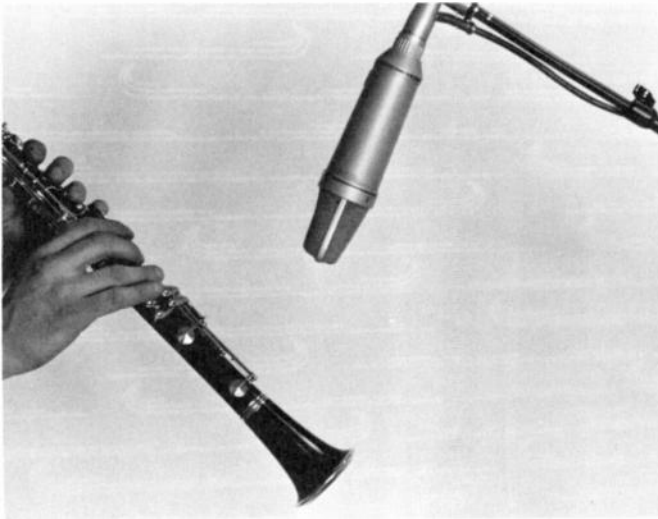
Figure 14.11. Woodwinds are best picked up by placing a mic near the finger holes.
