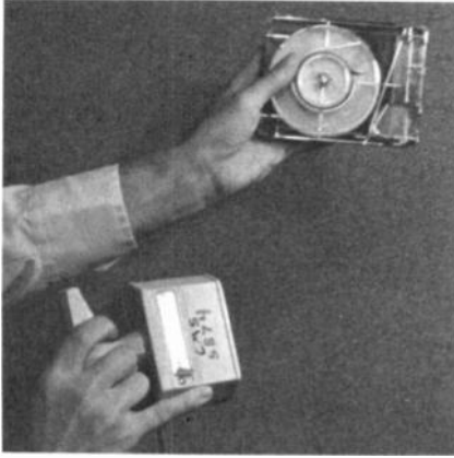
Figure 4.14. Move the bulker away from the cart gradually before you turn off the switch. If the magnetic field is suddenly turned off, it can impart a noise on the tape.
