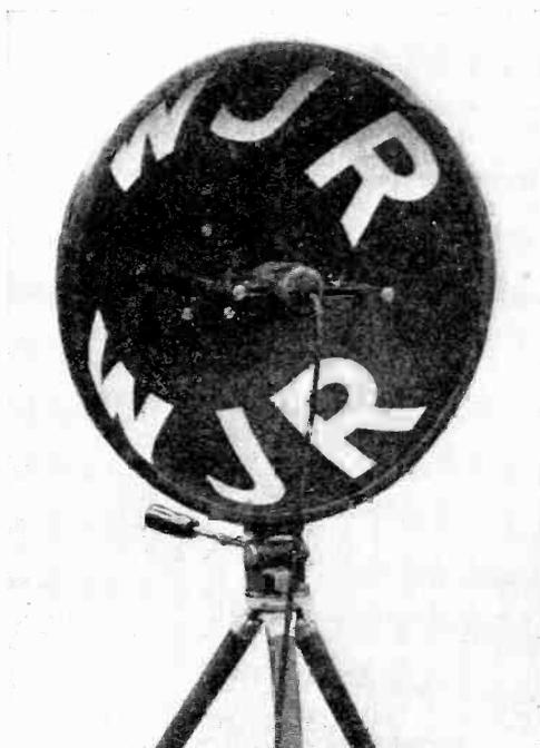
FIG. 12.—Improvised parabolic microphone.
